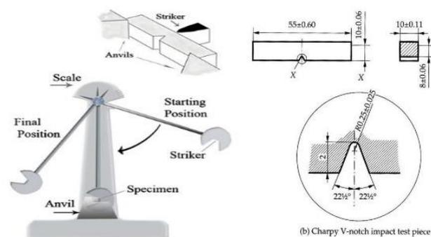
Fig. 20. Apparatus for impact testing of material
