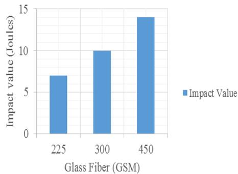
Fig. 21. Impact analysis of E-Glass/Epoxy polymer.
