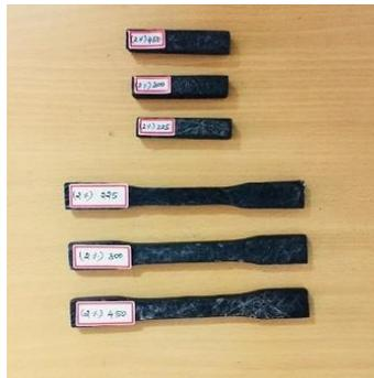
Fig. 15 Tensile and impact samples of pure Epoxy and E-fibre with 2.0 wt % of MWCNT &  $Al_2O_3$ .
