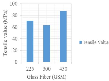
Fig. 16. Tensile analysis of E-Glass/Epoxy polymer.
