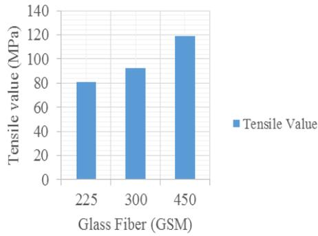
Fig. 18. Tensile analysis of 1.5wt% MWCNTs.
