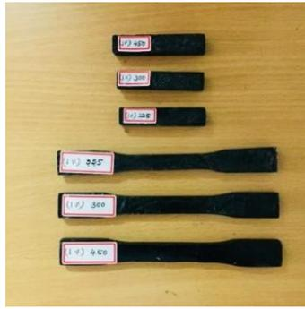
Fig. 13 Tensile and impact samples of pure Epoxy and E-fibre with 1.0 wt % of MWCNT &  $Al_2O_3$ .
