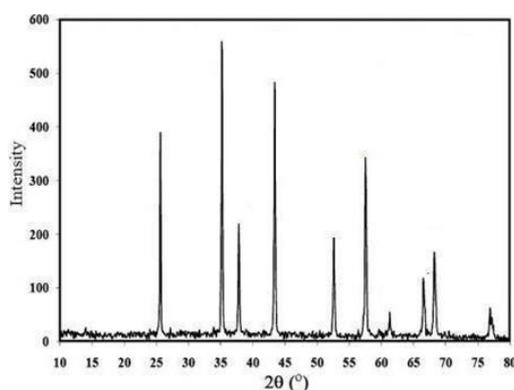
Fig. 9. X-Ray Diffraction (XRD) image of  $Al_2O_3$
