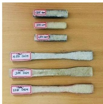
*Fig. 12. Tensile and impact samples of pure Epoxy and E-fibre.*
