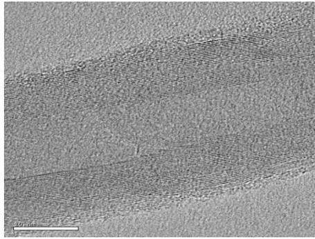
Fig. 3. Transmission electron microscopy image of MWCNTs (TEM).
