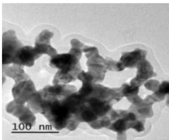
Fig. 7. Transmission Electron Microscopy image of  $\text{Al}_2\text{O}_3$  (TEM).
