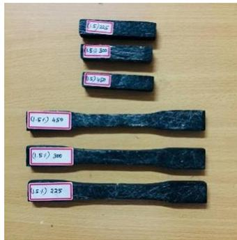
Fig. 14 Tensile and impact samples of pure Epoxy and E-fibre with 1.5 wt % of MWCNT &  $Al_2O_3$ .
