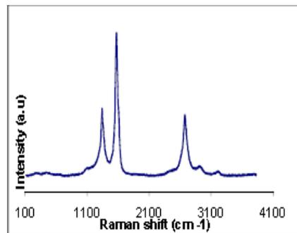
Fig. 5. Raman Spectrum Analysis of MWCNTs.
