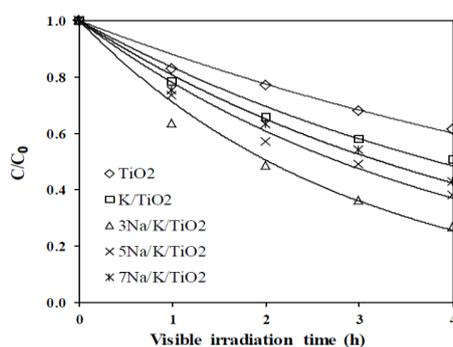
Fig. 5. Photocatalytic performance curves of  $\text{TiO}_2$  and composite films on degradation of MB under visible light irradiation.
