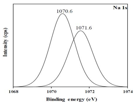
Fig. 4. The high-resolution XPS spectra of Na 1s on the surface of  $3\text{Na/K/TiO}_2$  thin film.
