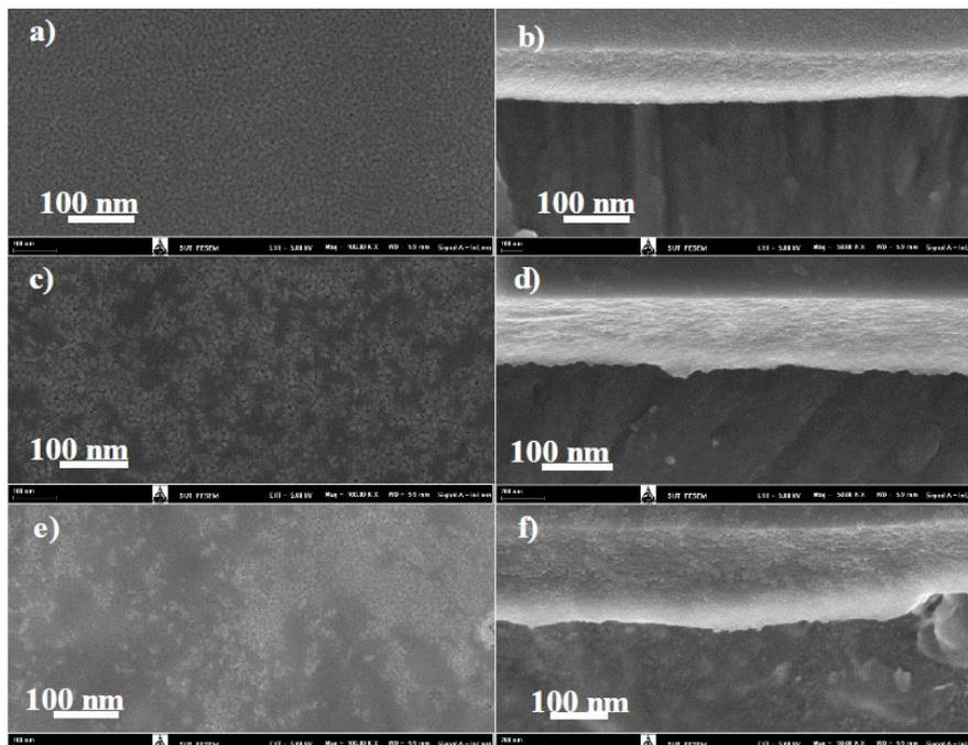
Fig. 1. FESEM images of (a) pure  $\text{TiO}_2$  and (b) cross-section, (c)  $\text{K/TiO}_2$  and (d) cross-section, (e)  $3\text{Na/K/TiO}_2$  and (f) cross-section films.
