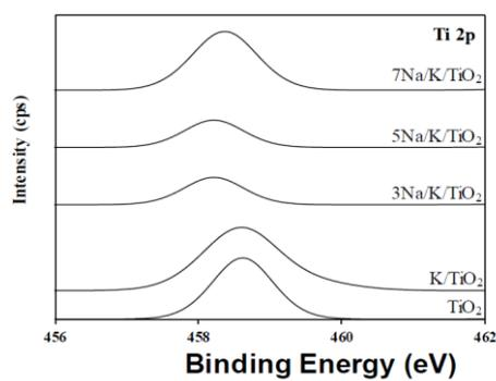
Fig. 2. XPS spectrum of Ti 2p on the surface of  $\text{TiO}_2$  and composite films.
