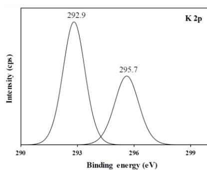
Fig. 3. The high-resolution XPS spectra of K 2p on the surface of  $3\text{Na/K/TiO}_2$  thin film.
