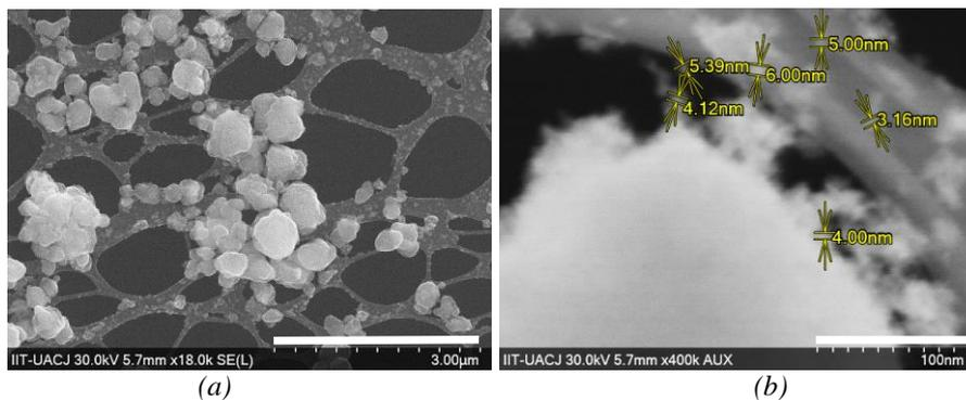
Fig. 5. SEM micrographs for TiO<sub>2</sub> nanoparticles.
