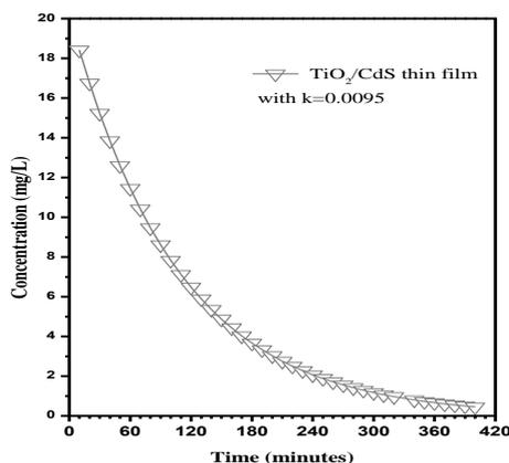
Fig. 10. Reaction kinetics of methylene blue degradation.
