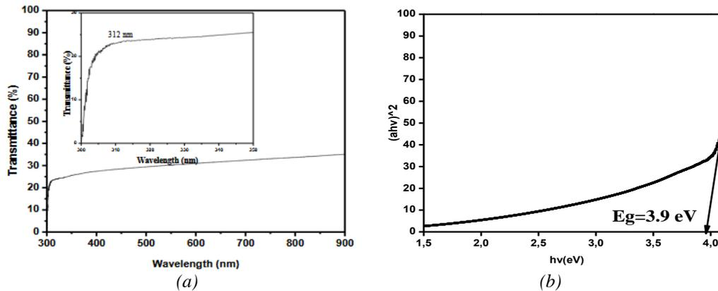
Fig. 4. (a) UV-Vis transmission spectra obtained for TiO<sub>2</sub> Nps thin film and (b) Tauc variable vs Energy.
