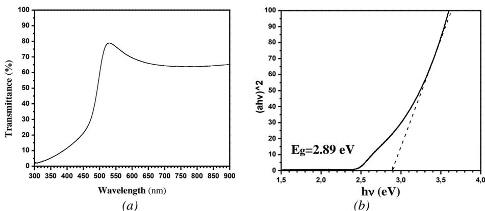
Fig. 1. (a) UV-Vis transmission spectra obtained for a CdS thin film deposited by CBD; (b) Tauc variable vs Energy.
