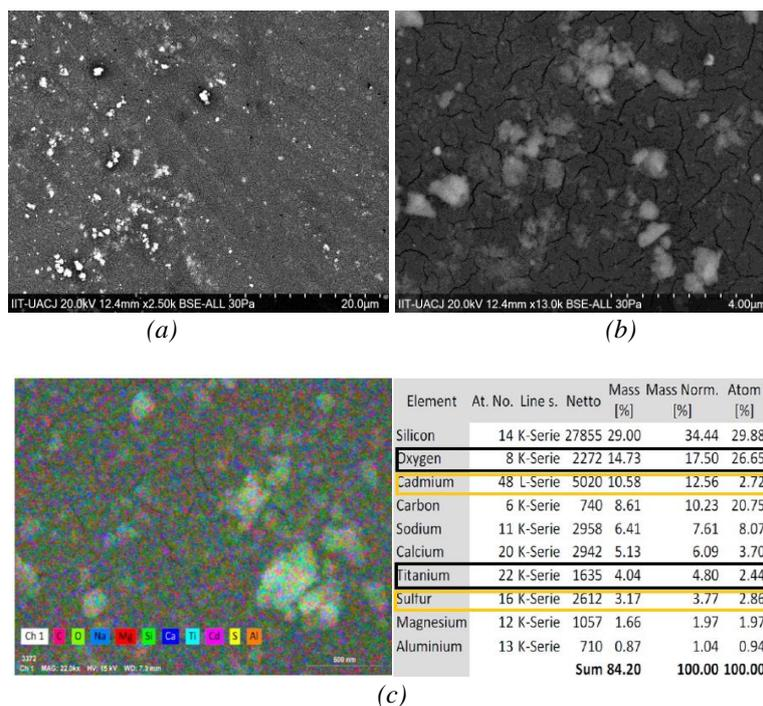
Fig. 8. (a) and (b) SEM micrographs and (c) EDAX analysis for  $\text{TiO}_2/\text{CdS}$  thin films.
