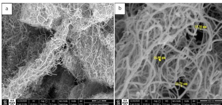
Fig. 2. (a, b) FE-SEM images of MW-CNT at different magnification.
