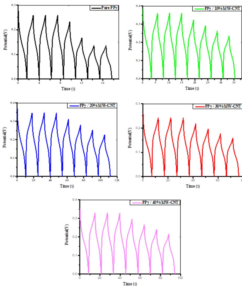
Fig. 6. Galvanostatic charge–discharge of PPy and PPy / MW-CNT electrode for supercapacitor.
