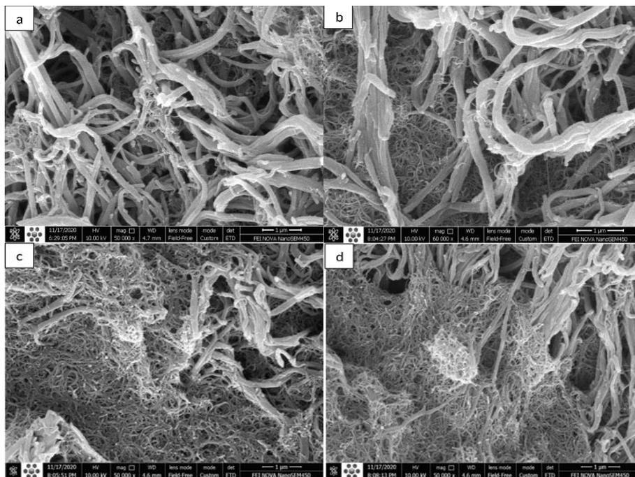
Fig. 3. (a, b, c, d) FE-SEM images of PPY / MW-CNT nanocomposites at different doping rates of CNT ( a- 10%, b-20%, c-30%, d-40% ).
