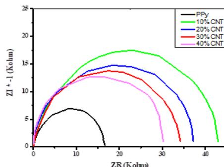
Fig. 8. Nyquist plots of the electrochemical impedance spectroscopy for the PPy, and PPy / MW-CNT.
