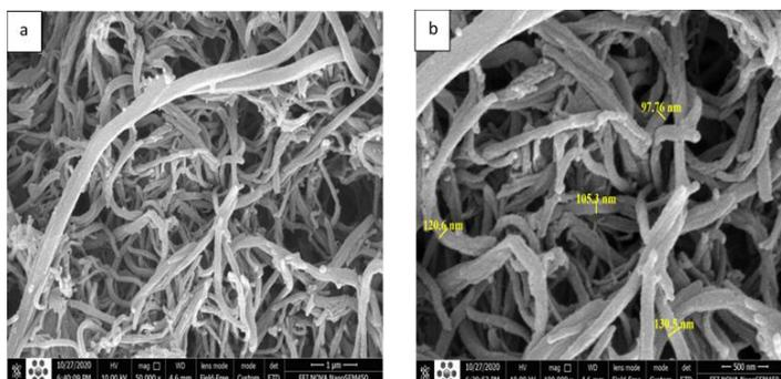
Fig. 1. (a , b) FE-SEM images of pure PPy nanofibers at different magnification.
