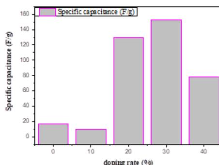
Fig. 5. Specific capacitance of the PPy/MW-CNT composite film at different doping rates.
