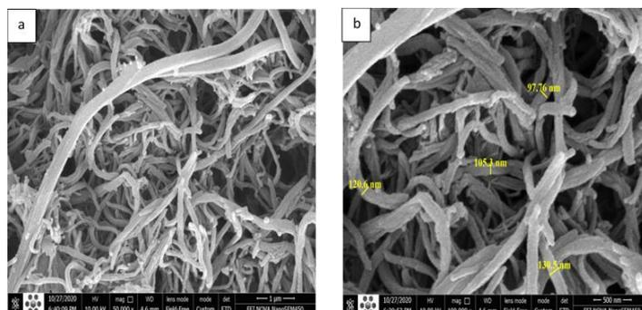
Fig. 1. (a , b) FE-SEM images of pure PPy nanofibers at different magnification.
