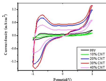
Fig. 4. CV curves of the PPY/MW-CNT composite film under different doping rate, at the scanning rate 5 mV s<sup>-1</sup>.
