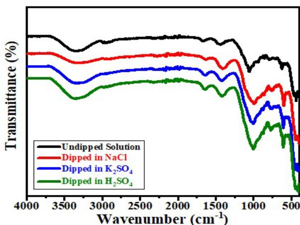
Fig. 1. FTIR spectra of fly ash geo-polymer samples.
