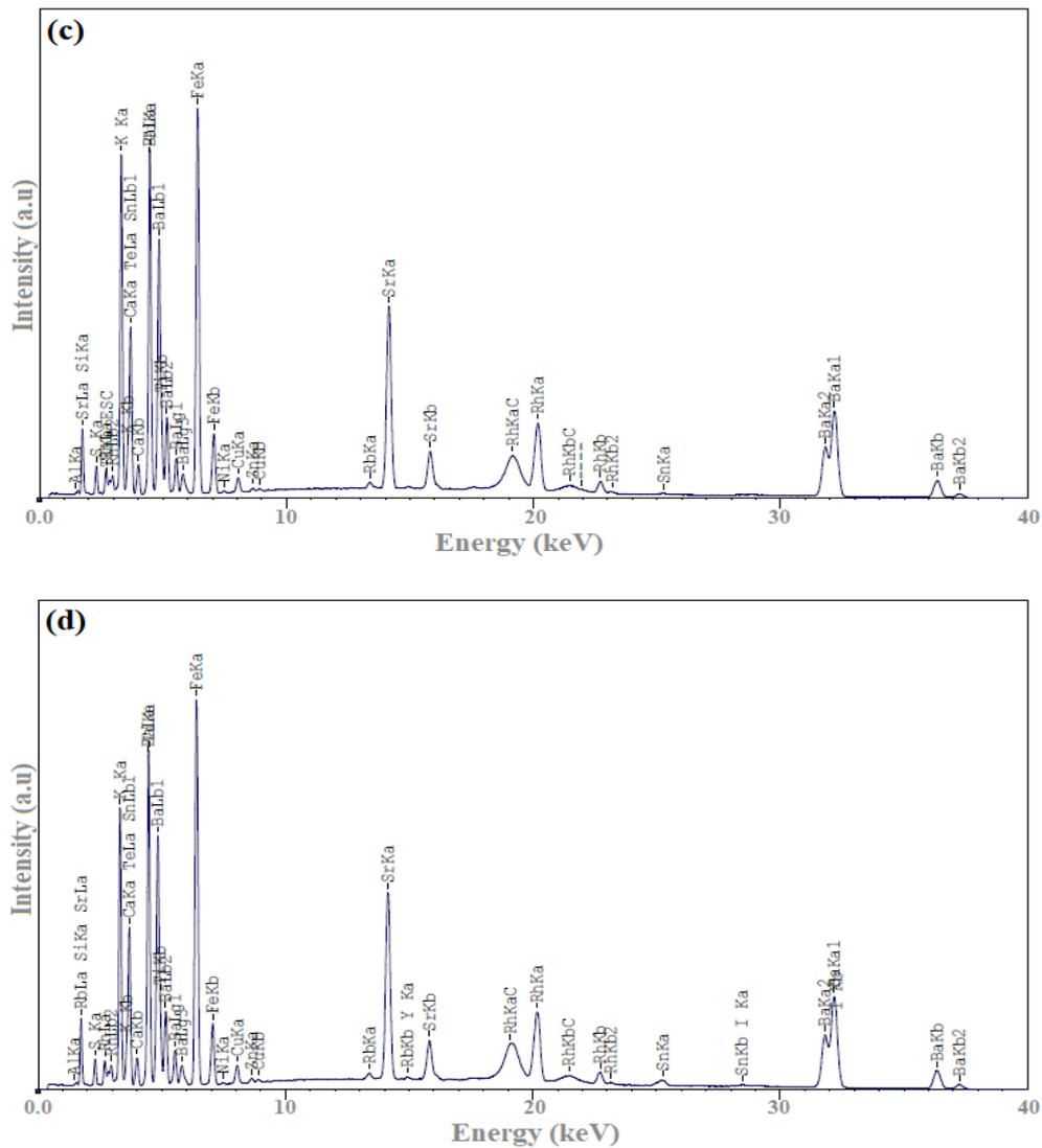
Fig. 3. XRF pattern of fly ash geo-polymer samples, (a) Undipped solution, (b) Dipped in NaCl, (c) Dipped in K<sub>2</sub>SO<sub>4</sub>, and (d) Dipped in H<sub>2</sub>SO<sub>4</sub>.
