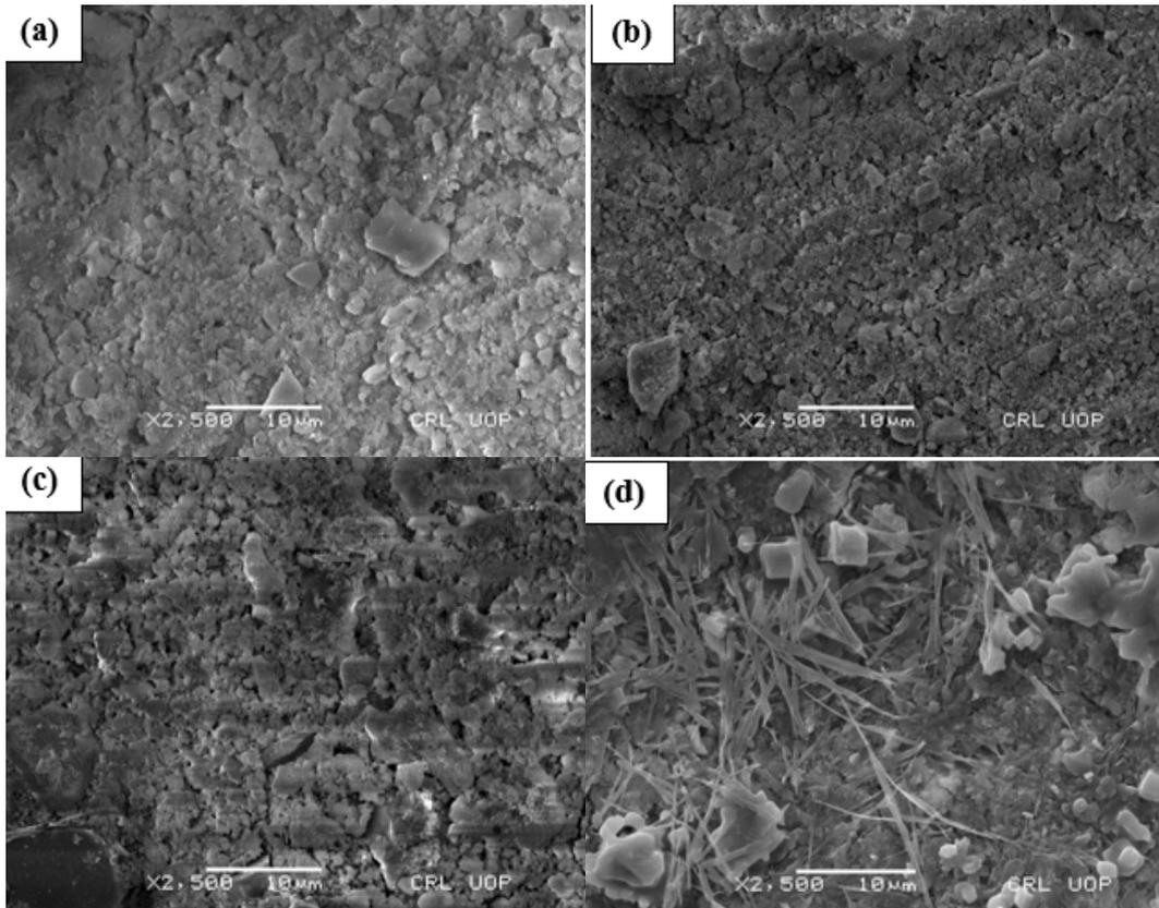
Fig. 4. SEM images of fly ash geopolymer samples, (a) Undipped solution, (b) Dipped in NaCl, (c) Dipped in  $K_2SO_4$ , and (d) Dipped in  $H_2SO_4$ .
