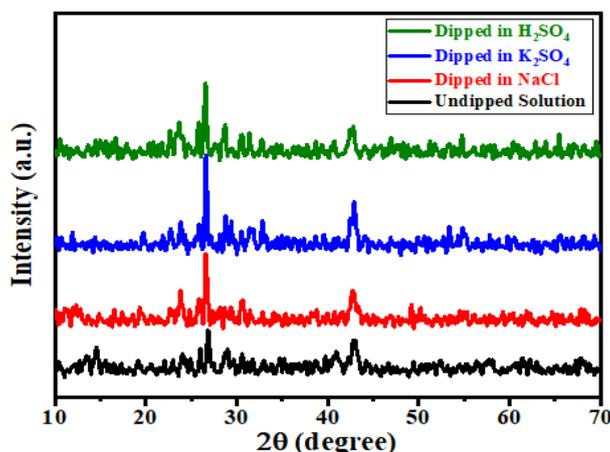
Fig. 2. XRD pattern of the fly ash geo-polymer samples.
