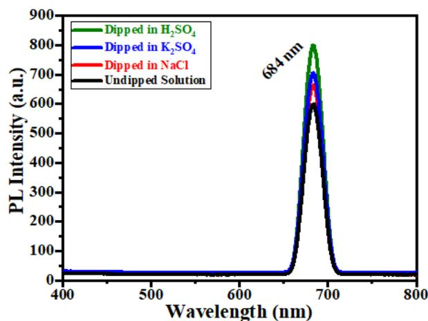
Fig. 5. The PL spectra of all samples, (a) Undipped solution, (b) Dipped in NaCl, (c) Dipped in  $K_2SO_4$ , and (d) Dipped in  $H_2SO_4$ .
