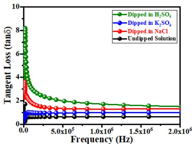
Fig. 7. The variation of tangent loss with frequency of the fly ash geopolymer.
