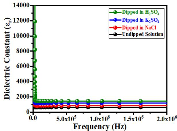
Fig. 6. The variation of dielectric constant with frequency of the fly ash geopolymer.
