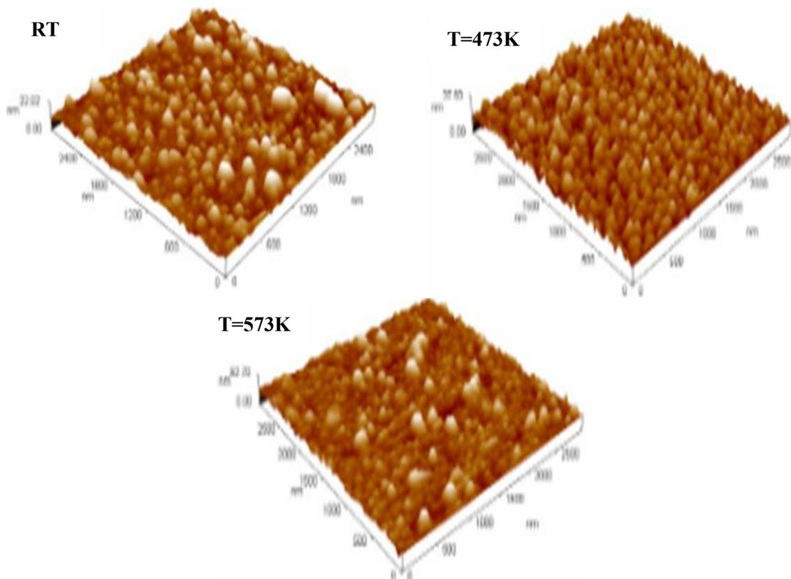
Fig. 2. 3D (AFM) of thin films AIS at R.T and (473,573) K.
