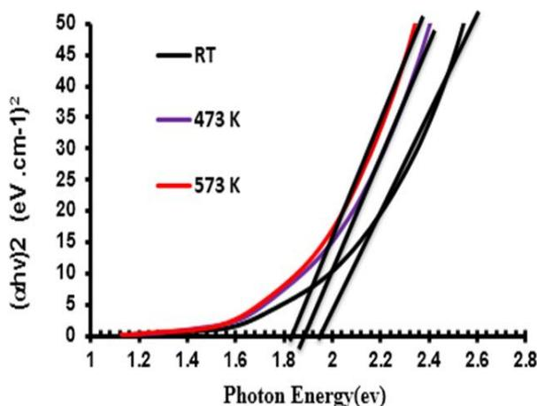
Fig. 5.  $(\alpha hv)^2$  vs.  $hv$  plot of as prepared of thin films AIS at R.T and (473,573) K.
