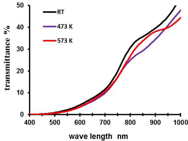
Fig. 3. Transmittance spectra vs. wave length of thin films AIS at R.T and (473,573) K.
