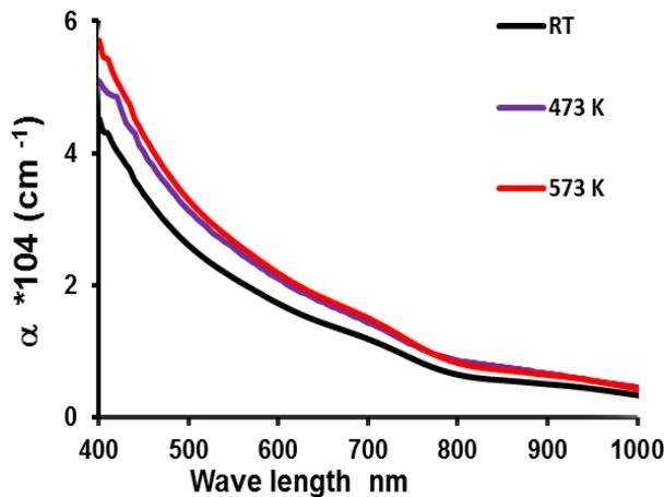
Fig. 4. The  $\alpha$  vs. Wavelength of as prepared AIS at R.T and (473,573) K.
