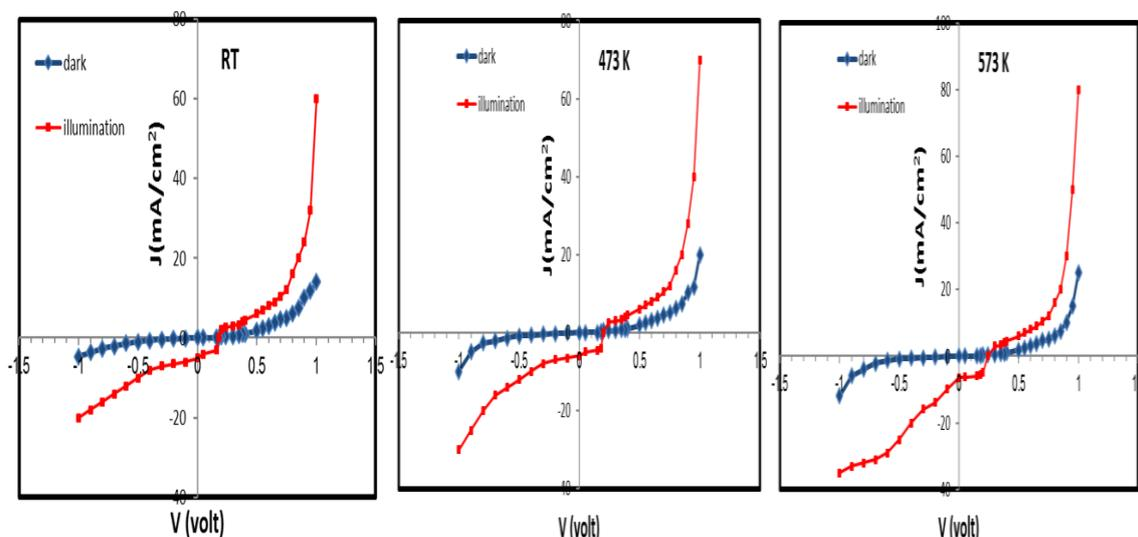
Fig. 6. I-V characteristic for AIS/Si under illumination and dark solar cell AIS at R.T and (473,573) K.
