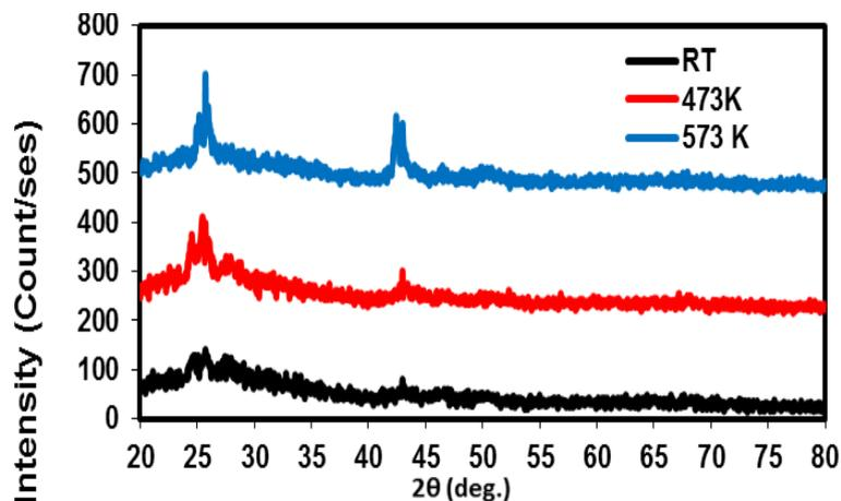
Fig. 1. XRD pattern for thin film AIS at R.T and (473,573) K.
