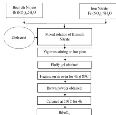
Fig. 1. Synthesis process of  $\text{BiFeO}_3$ .
