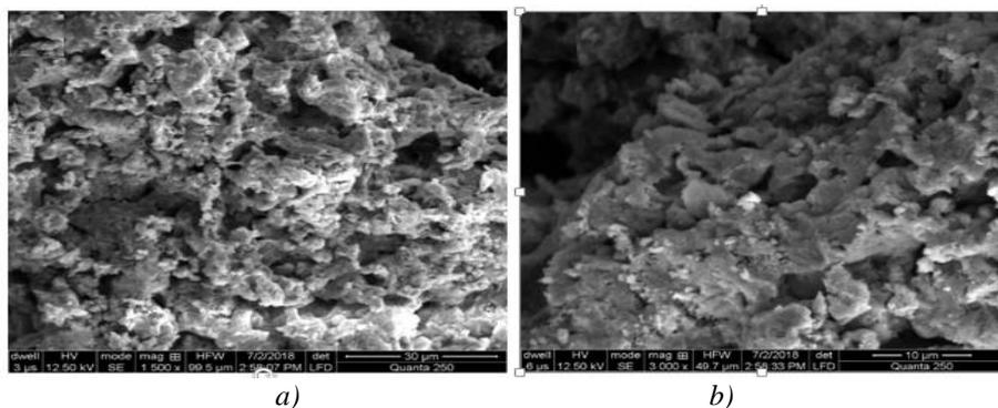
Fig. 4. SEM analysis of bismuth ferrite (BiFeO<sub>3</sub>) nanoparticles at (a) 1500x (b) 3000x.
