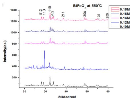
Fig. 2. XRD graph of BiFeO<sub>3</sub> with different chemical concentrations at 550°C.
