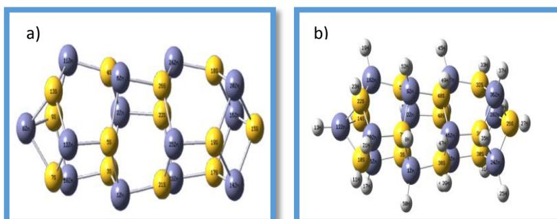
Fig. 2. The wurtzoid of ZnS nanotubes structure a) bare and b) H-passivated after optimization.
