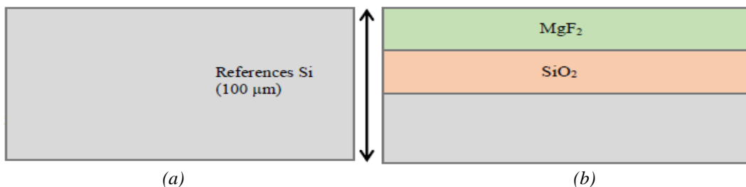
Fig. 1. (a) Reference: Schematic diagrams of Light Trapping schemes in silicon solar cells without anti reflective coatings (as a reference) for planar solar cells; (b) \text{MgF}_2 ARC for Si solar cell with thickness of 75 nm.
