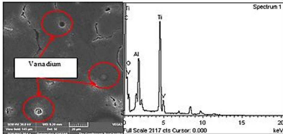
Fig. 2. SEM micrograph of a) sintered Ti-6V composites(b) corresponding EDAX spectrum.
