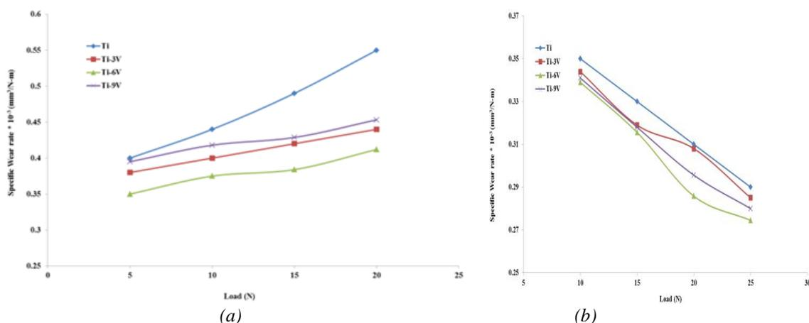
Fig. 3. Specific wear rate of Ti-V composites a) Load Vs SWR and b) SV Vs SWR.
