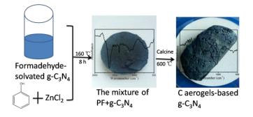
*Fig. 1. The process of the C aerogels-based* g- $C_3N_4$  *photocatalyst.*
