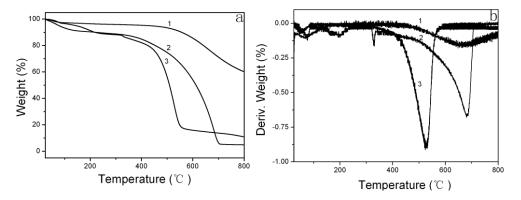
Fig. 5. TGA (a) and DTG (b) curves of the mixture of PF and  $g-C_3N_4$  (1),  $g-C_3N_4$  (2) and PF (3).
