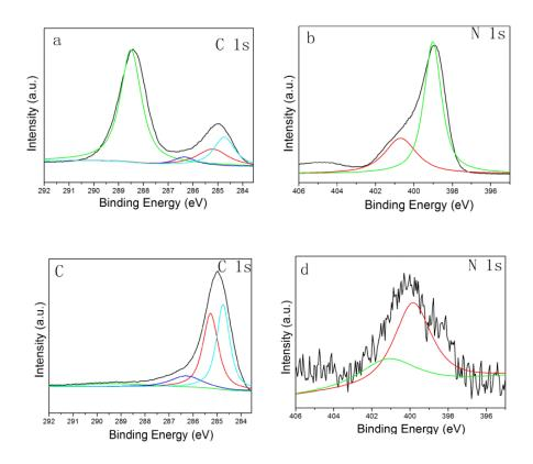
Fig. 3. XPS patterns (a) C 1s and (b) N 1s of g-C<sub>3</sub>N<sub>4</sub> and (c) C 1s and (d) N 1s of C aerogels-based g-C<sub>3</sub>N<sub>4</sub>.
