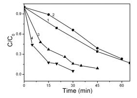
Fig. 9. Photocatalytic degradation of g- $C_3N_4(1)$ , C aerogels-based g- $C_3N_4(0.1)(2)$ , C aerogels-based g- $C_3N_4(0.2)(3)$ , C aerogels-based g- $C_3N_4(0.3)(4)$ .
