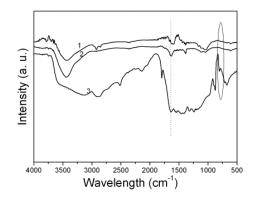
Fig. 2. FTIR spectra of (1) C aerogels-based g-C<sub>3</sub>N<sub>4</sub>, (2) C and (3) g-C<sub>3</sub>N<sub>4</sub>.
