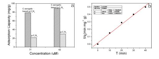
Fig. 8. (a) Adsorption capacity of samples; (b) Pseudo second order kinetics of C aerogels-based g-C<sub>3</sub>N<sub>4</sub>.
