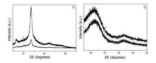
Fig. 4. XRD spectra of (a)  $g-C_3N_4$  (1) and  $g-C_3N_4$  (a); (b) C (1) and C aerogels-based  $g-C_3N_4$  (2).
