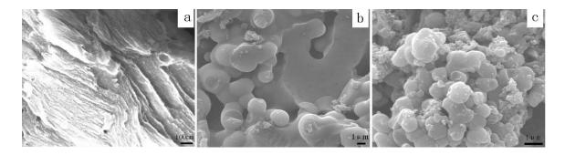
Fig. 7. SEM of g- $C_3N_4$  (a), C (b) and C aerogels-based g- $C_3N_4$  (c).
