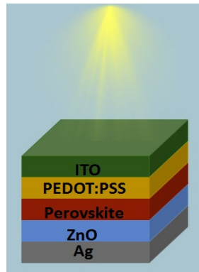
Fig. 7. Layer arrangements of perovskite solar cell.
