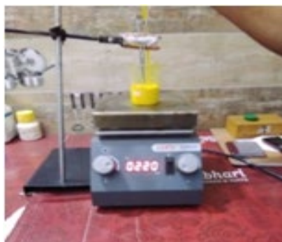
Fig. 1. Experimental arrangement of CdZnS films by CBD method.
