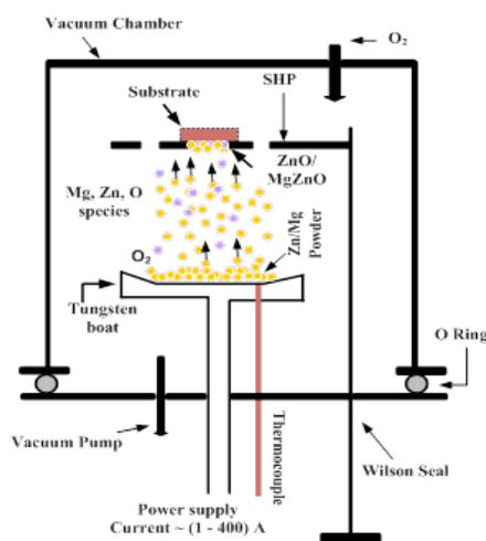
*Fig. 1. Schematic diagram of thermal evaporator used to synthesize un-doped ZnO and Mg-doped ZnO TFs.*
