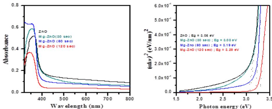
Fig. 7. The change in absorption edge (A) and the  $E_g$  values (B) of ZnO and Mg-doped ZnO TFs synthesized for different exposure time of ZnO in Mg contents.
