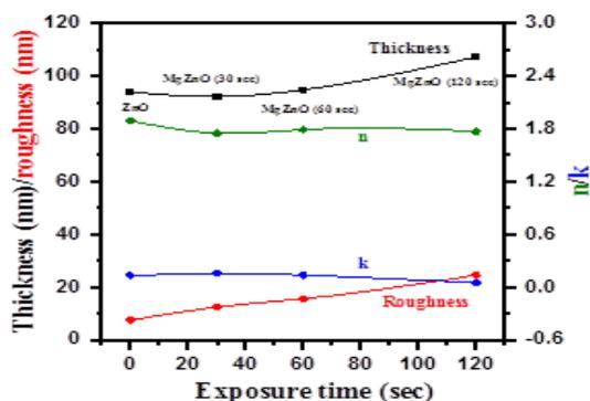
Fig. 6. Variation in film thickness, roughness, refractive index and extinction coefficient as function of exposure time of un-doped ZnO in Mg contents.
