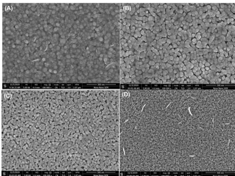
Fig. 4. SEM microstructures of (A) un-doped ZnO and (B), (C), (D) Mg-doped ZnO TFs.
