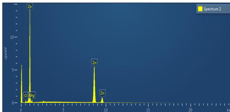
Fig. 5. Typical EDX spectrum of Mg-doped ZnO TF.
