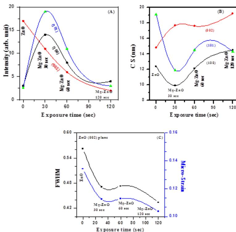
Fig. 3. Variation in (A) peak intensities, (B) C S of (100), (002), (101) plane, (C) FWHM and micro-strains developed in (002) plane of un-doped ZnO and Mg-doped ZnO TFs.
