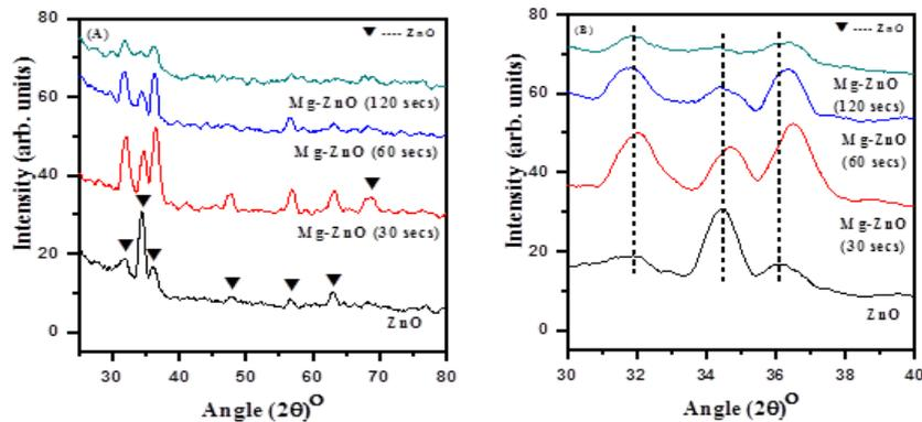
Fig. 2. XRD patterns of (A) un magnified ZnO, Mg-ZnO and (B) magnified Mg-ZnO TFs.
