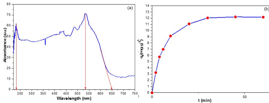
Fig. 4. (a) Absorbance spectrum for visible light by BiOI and (b) The contact time investigation for the adsorption of MG on BiOI.
