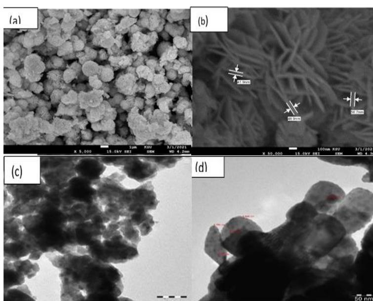
Fig. 2. (a)-(b) SEM results, and (c)-(d) TEM results for the prepared BiOI.
