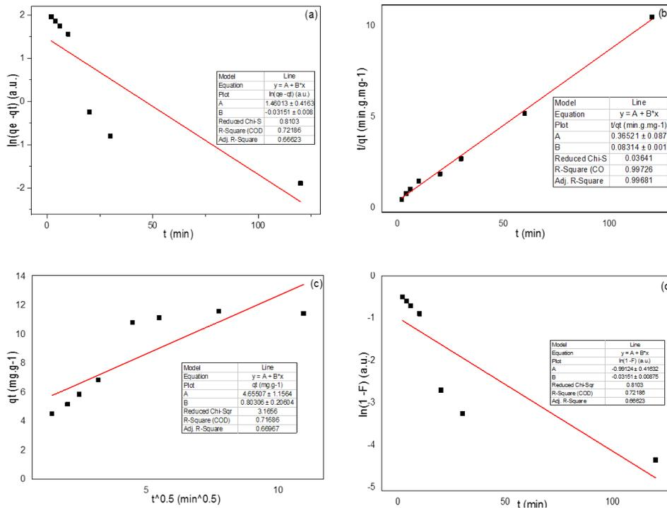
Fig. 5. (a) pseudo-first-order model, (b) pseudo-second-order model, (c) intraparticle-diffusion model and (d) liquid-film-diffusion model kinetic investigations for the MG adsorption on BiOI.
