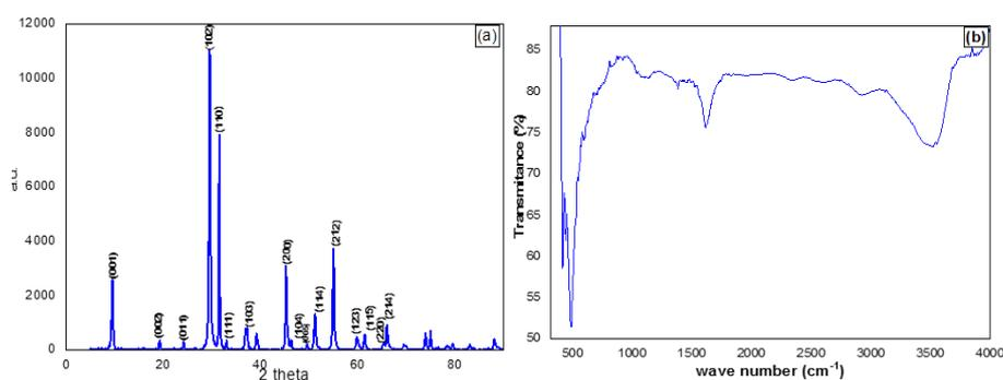
Fig. 1. (a) XRD pattern and (b) FTIR analysis for the prepared BiOI photocatalyst.
