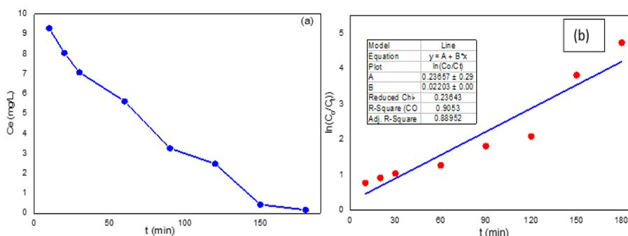
Fig. 6. (a) degradation trend and (b) 1st-order kinetic investigation for the MG photocatalytic degradation under sunlight by BiOI-photocatalyst.
