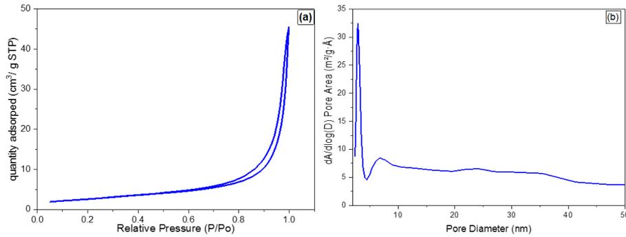
Fig. 3. (a) Nitrogen adsorption-desorption isotherm and (b) pore size distribution for BiOI.
