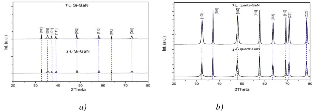
Fig. 1. XRD pattern of GaN thin films deposited with different number of coatings layers onto (a) silicon 7 and 3 layers, (b) quartz 7 and 3 layers.
