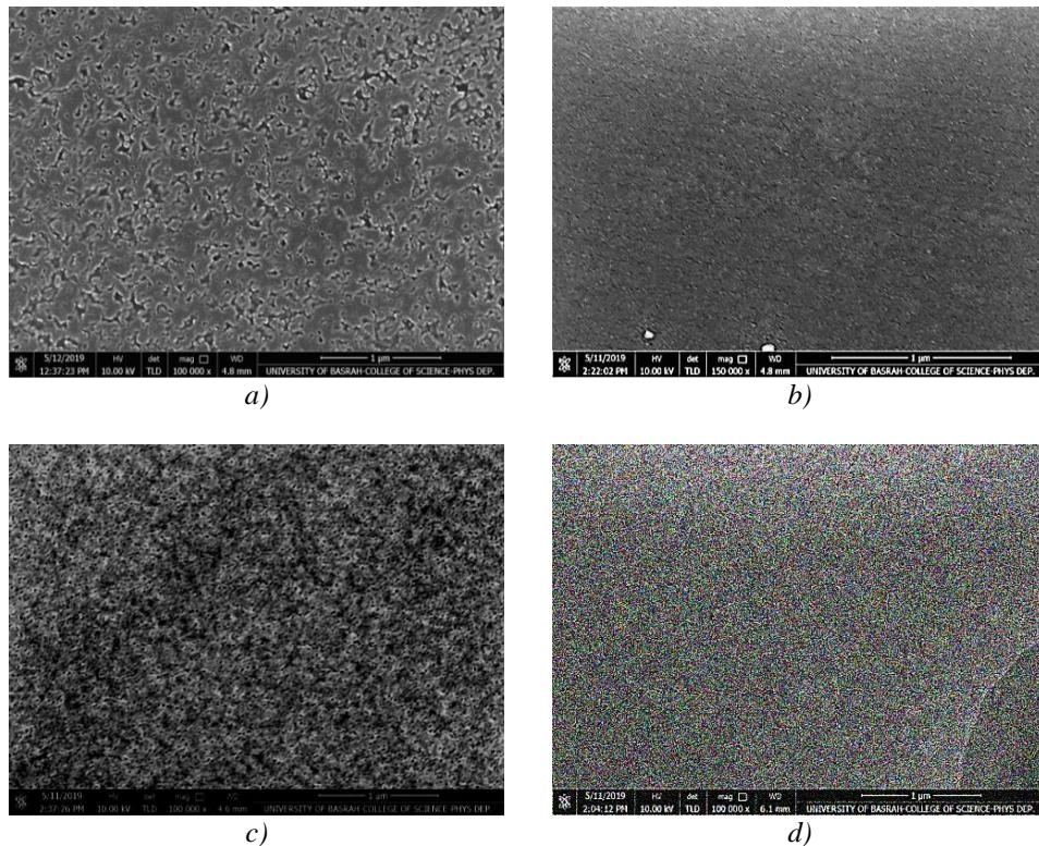
*Fig. 2. FESEM image of GaN thin films deposited with different number of coatings onto
