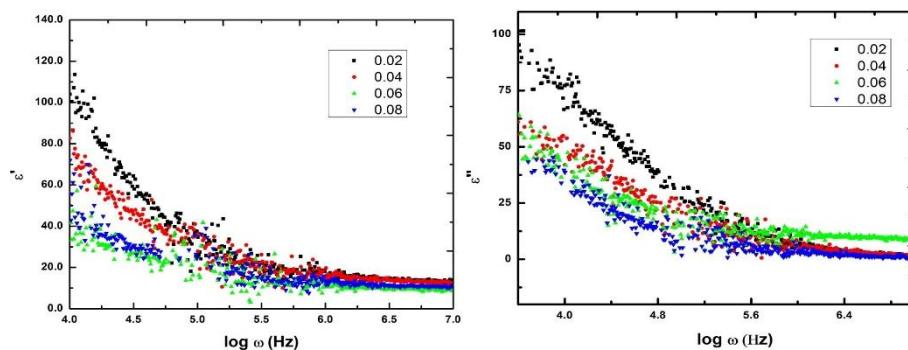
Fig. 4. Frequency dependence of dielectric constant ( $\epsilon'$ ), and dielectric loss ( $\epsilon''$ ).
