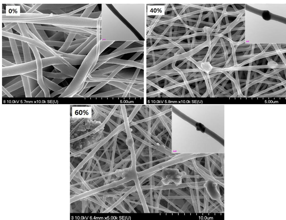
Fig. 4 FE-SEM images of (a) Pristine PU, (b) PU/FAP 40wt%, and (c) PU/FAP 60 wt%
