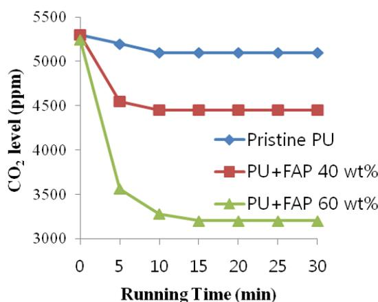
Fig. 8 Experimental CO<sub>2</sub> evaluation results of different mats (a) Pristine PU, (b) PU+FAP 40wt%, and (c) PU+FAP 60 wt%
