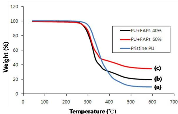
Fig.7 TGA curves of different mats (a) Pristine PU, (b) PU+FAP 40wt%, and (c) PU+FAP 60 wt%
