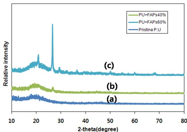
Fig.5 XRD spectra of (a) pristine PU, (b) PU+FAP 40 wt%, and (c) PU+FAP 60 wt%
