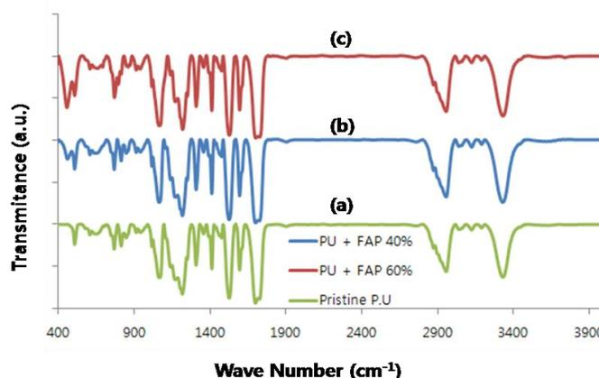
Fig. 6 FTIR spectra of different mats (a) Pristine PU, (b) PU+FAP 40wt%, and (c) PU+FAP 60 wt%
