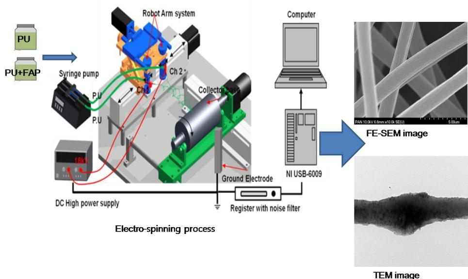
Fig. 1 Schematic of experiment equipment
