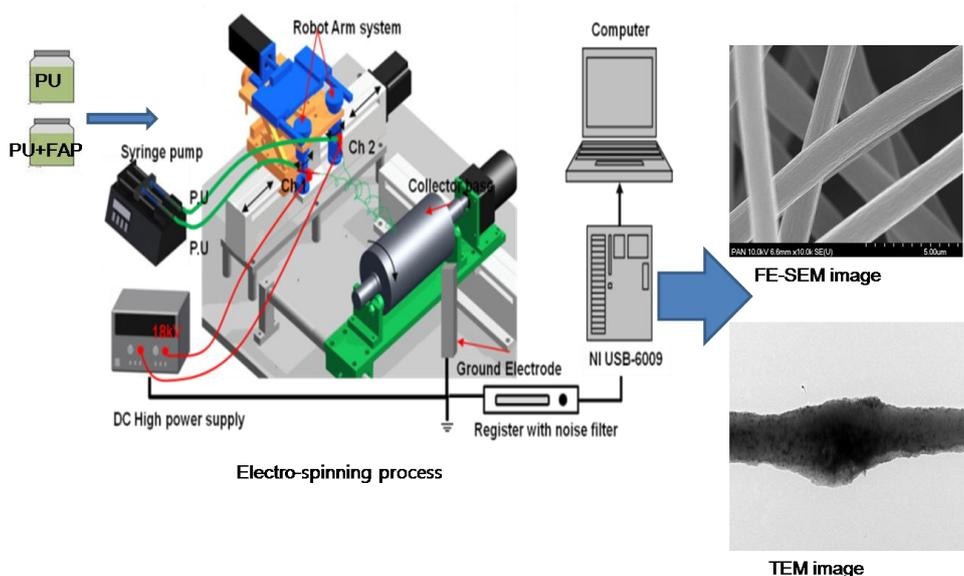
Fig. 1 Schematic of experiment equipment
