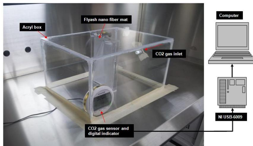
Fig. 3 Real experiment configuration and DAQ flowchart
