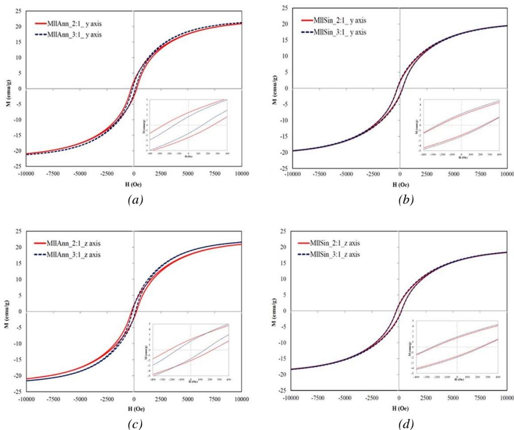
Fig. 4. *M-H* curves of MnBi/Co magnets prepared by using a) annealed and b) sintered powders with Mn:Bi ratio of 2:1 and 3:1 and aligned in magnetic field parallel to the sample's plane (y-axis); c) annealed and d) sintered powders with Mn:Bi ratio of 2:1 and 3:1 and aligned in magnetic field perpendicular to the sample's plane (z-axis). Insets are magnified portions at low fields up to  $\pm 400$  Oe.
