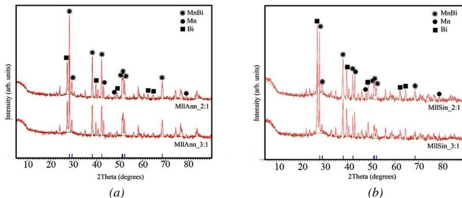
Fig. 1. XRD patterns of (a) annealed and (b) sintered samples prepared with Mn:Bi ratio of 2:1 and 3:1 after the ball-milling.
