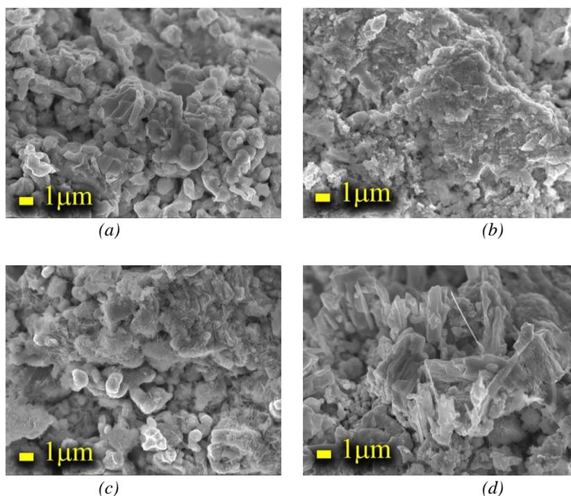
*Fig. 3. FESEM images of MnBi/Co magnets from annealed samples prepared with Mn:Bi ratio of a) 2:1 and b) 3:1; sintered samples prepared with Mn:Bi ratio of c) 2:1, d) 3:1.*
