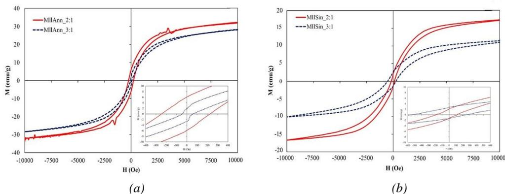
Fig. 2. *M-H* curves of (a) annealed and (b) sintered samples prepared with Mn:Bi ratio of 2:1 and 3:1 after the ball-milling. Insets are magnified portions at low fields up to  $\pm 400$  Oe.
