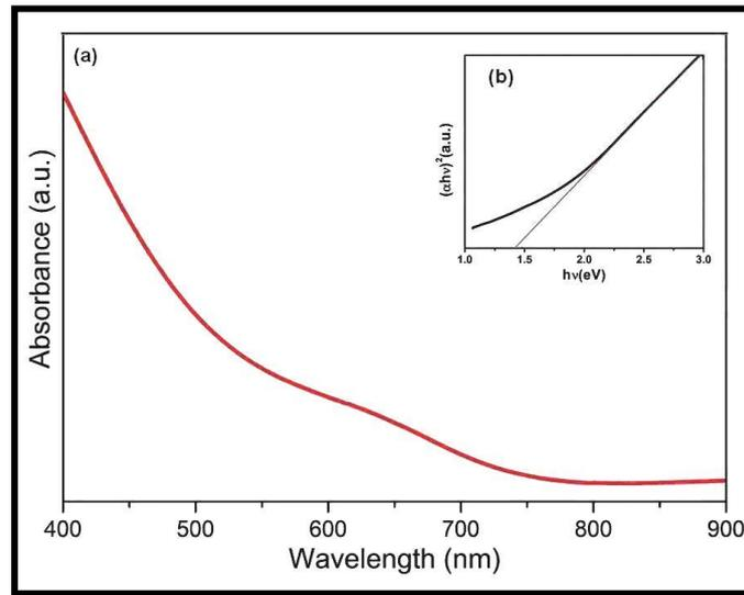
Fig.3 (a) UV-Visible absorption spectrum of SnS films and (b) Plot of  $(ah\nu)^2$  Vs photon energy
