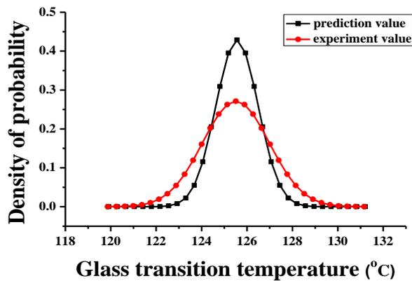
Fig. 3 The comparison of the TMA glass transition temperatures for prediction and the confirmation experiment
