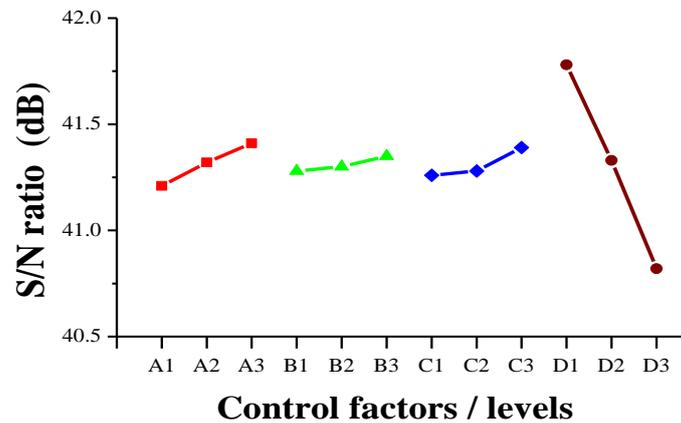
Fig 1 S/N factor response graph for the TMA glass transition temperature
