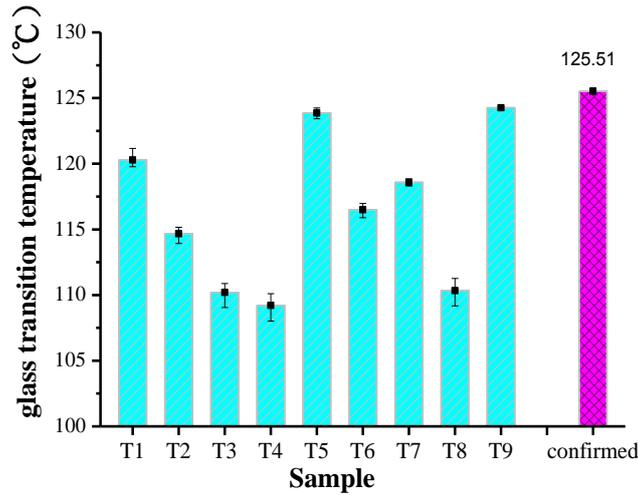
Fig. 2 The comparison of the TMA glass transition temperatures from different sample and the confirmation experiment
