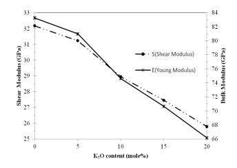
Fig. 2. Bulk modulus and Shear modulus versus  $K_2O$  content in 50TVKx glasses.
