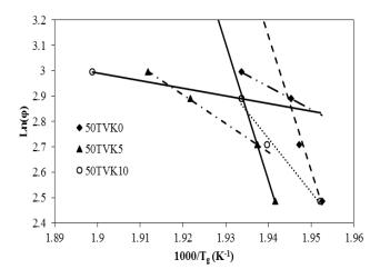
Fig. 6 Plots of Ln $\varphi$  versus 1000/Tg (Eq. 10) for 50TVKx glasses; straight lines are drawn for the guide for eye to distinct the different heating rate regions, and the slopes are equal to  $(-\Delta H^*/1000 R)$
