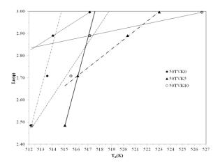
Fig. 5. Plots of  $T_g$  versus  $Ln \varphi$  for  $50TeO_2$ - $(50-x)V_2O_5$ - $xK_2O$  (x = 0, 5 and 10) glasses. The solid and dashed lines represent fit to Eq. (9) at different heating rate regions
