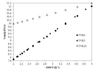
Fig. 9. Calculated viscosity as a function of 1000/T in the glass transition region for 50TVKx glasses (logarithmic function on the y-axis is in the base 10)
