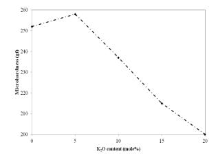
Fig. 3. Microhardness versus K<sub>2</sub>O content in 50TVKx glasses.
