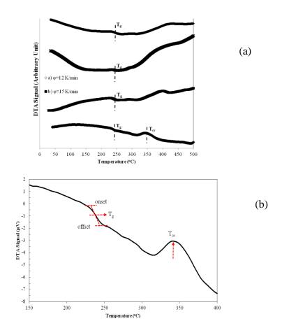
Fig. 4. a) DSC curves in 50TVK0 glass in different heating rates: a)  $\varphi = 12$  K/min, b)  $\varphi = 15$  K/min, c)  $\varphi = 18$  K/min and d)  $\varphi = 20$  K/min. b) A typical heating flow vs. temperature curve for a  $50TeO_2-50V_2O_5$ , mol%, glass at a heating rate of 12 K/min
