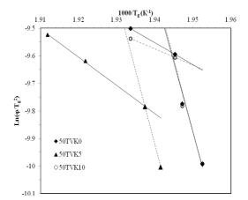
Fig. 6 Kissinger plots  $Ln(\frac{\varphi}{T_g^2})$  of versus 1000/ $T_g$  for 50TVKx glasses (x = 0, 5 and 10)
