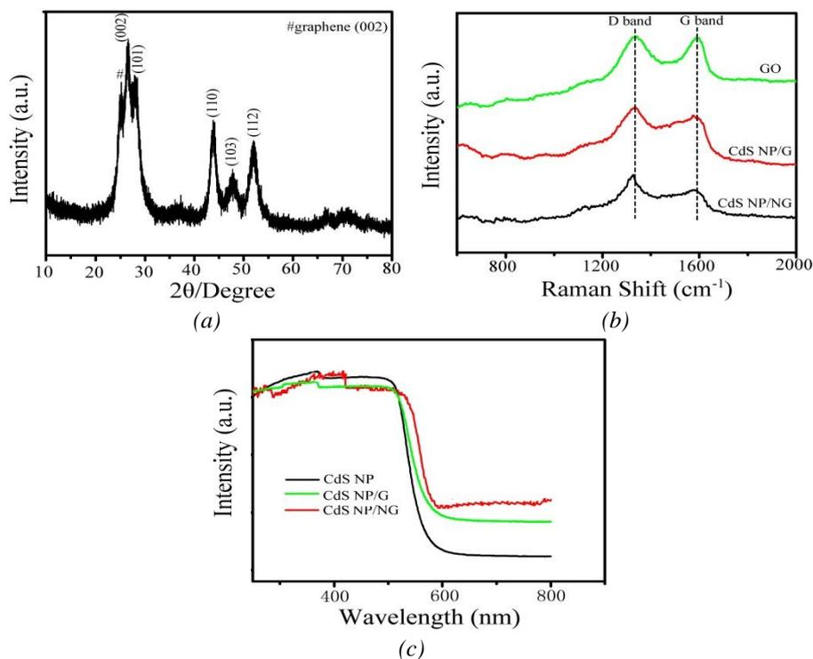
Fig. 1. (a)XRD, (b)Raman spectra, (c) UV/Vis diffuse reflectance spectra of the composites.
