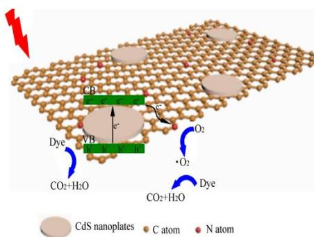
Fig. 6. Proposed photocatalytic mechanism of CdS NP/NG.
