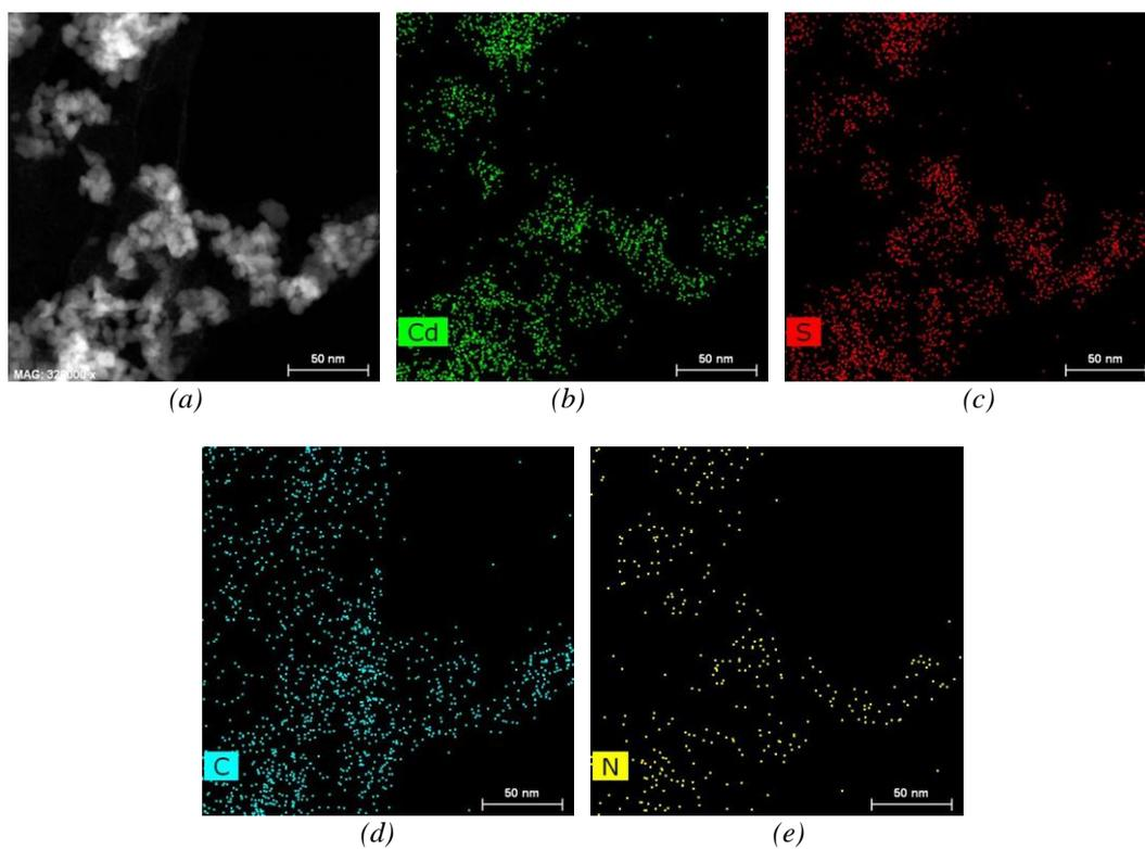
Fig. 4. (a) TEM of EDS mapping of selected area, (b) element Cd mapping, (c) element S mapping, (d) element C mapping, (e) element N mapping of CdS NP/NG.
