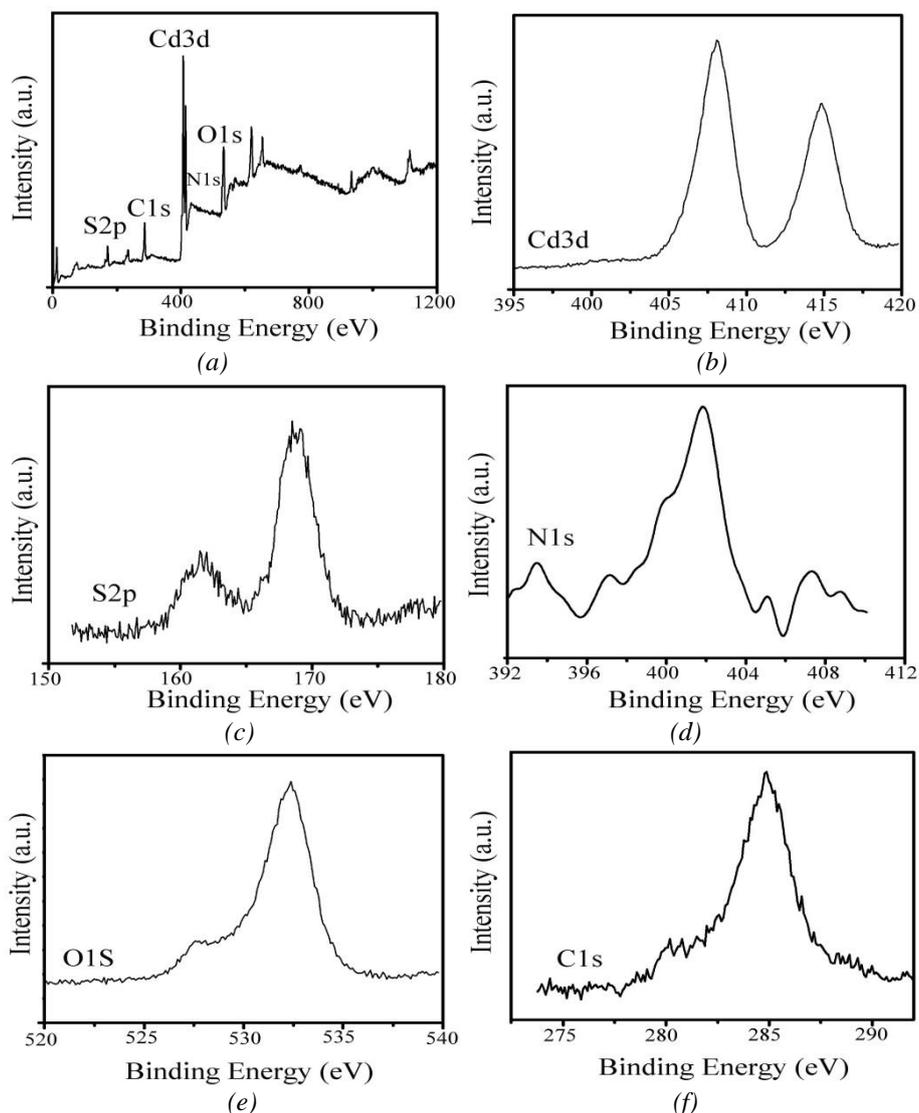
Fig. 2. Typical XPS spectra of the CdS NP/NG composite: (a) survey spectra, (b) Cd 3d region XPS spectrum, (c) S 2 p region XPS spectrum, (d) N 1s s region XPS spectrum, (e) O1s region XPS spectrum, (f) C1s region XPS spectrum.
