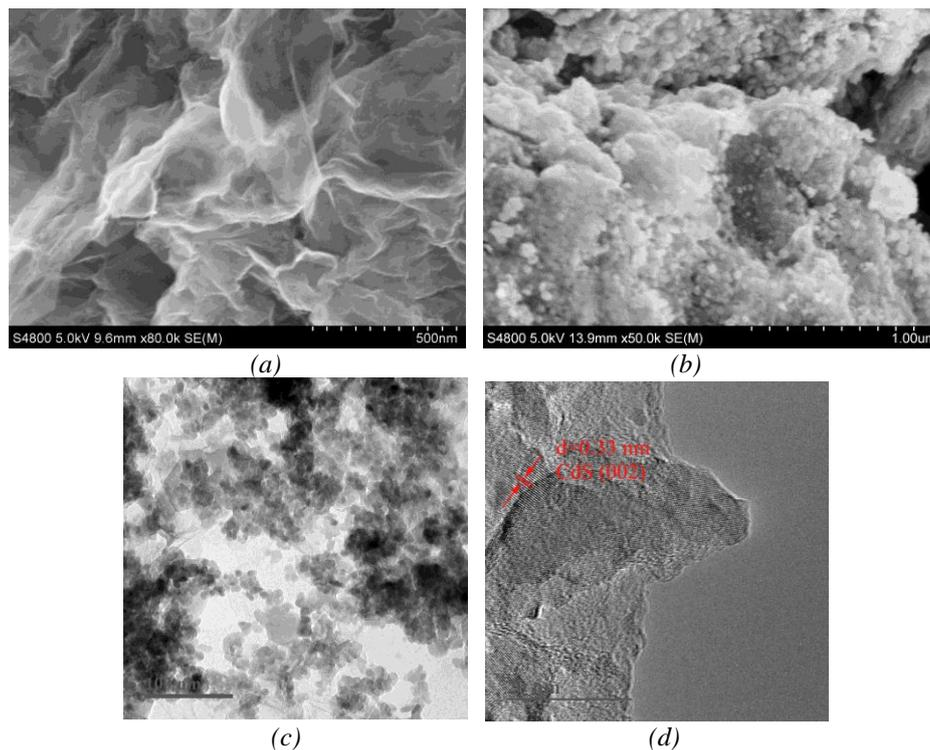
Fig. 3. (a)SEM of graphene, (b) SEM, (c)TEM, (d)HRTEM images of CdS NP/NG.
