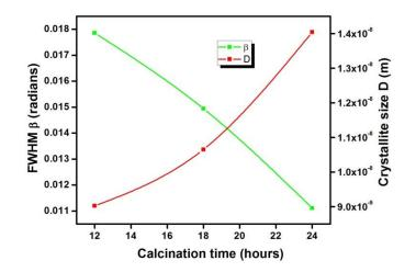
Fig. 3 Variations of FWHM and crystallite size as a function of calcination time for MgAl<sub>2</sub>O<sub>4</sub> thin films
