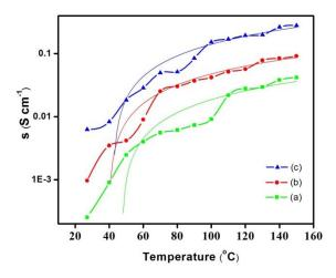
Fig. 10 Electrical conductivity variations for different time calcined  $M_gAl_2O_4$  thin films
