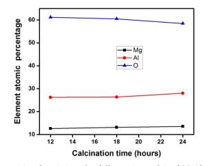
Fig. 12 Compositional variations for different time calcined MgAl<sub>2</sub>O<sub>4</sub> thin films
