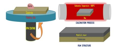
Scheme 1 Schematic diagram of film preparation processes and film structure
