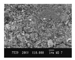
Fig. 11(c) SEM micrograph of  $500^{\circ}C$  calcined  $M_{gAl_2O_4}$  thin film at 24 hours
