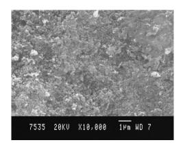
Fig. 11(a) SEM micrograph of  $500^{\circ}C$  calcined  $M_{g}Al_{2}O_{4}$  thin film at 12 hours
