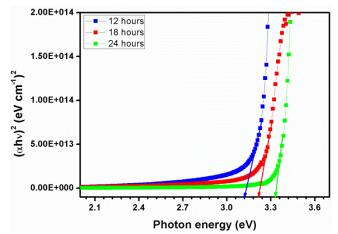
Fig. 7 Variations of Tauc's plot for various time calcined MgAl<sub>2</sub>O<sub>4</sub> thin films
