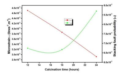
Fig. 4 Variations of micro strain and stacking fault probability as a function of calcination time for MgAl<sub>2</sub>O<sub>4</sub> thin films
