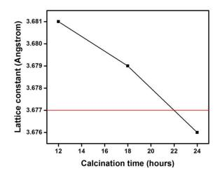
Fig. 2 Lattice constants variations of different time calcined MgAl<sub>2</sub>O<sub>4</sub> thin films
