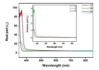
Fig. 9 Complex dielectric constants variations for different time calcined MgAl<sub>2</sub>O<sub>4</sub> thin films
