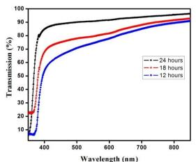
Fig. 6 Optical transmission variations as function of wavelength for different time calcined MgAl<sub>2</sub>O<sub>4</sub> thin films
