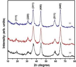
Fig. 1 X-ray diffraction patterns of various time calcined MgAl<sub>2</sub>O<sub>4</sub> thin films (a) 12 (b) 18 and (c) 24 hours
