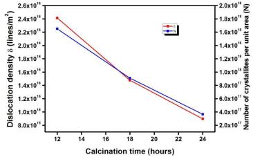
Fig. 5 Variations of dislocation density and number of crystallites per unit area as a function of calcination time for MgAl<sub>2</sub>O<sub>4</sub> thin films
