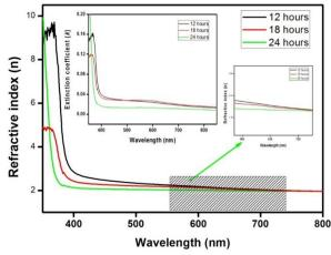
Fig. 8 Refractive indices variations for different time calcined  $MgAl_2O_4$  thin films
