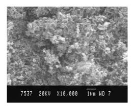
Fig. 11(b) SEM micrograph of  $500^{\circ}C$  calcined  $M_{g}Al_{2}O_{4}$  thin film at 18 hours
