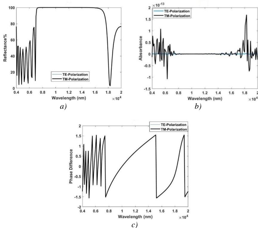
Fig. 2. (a) Reflectance, (b) Absorbance, and (c) Phase Difference as a function of the wavelength of coatings  $n_H = 5.64$ ,  $n_l = 1.44$ , and  $n_s = 5.64$ , for eight layers at an incident angle ( $0^\circ$ ).
