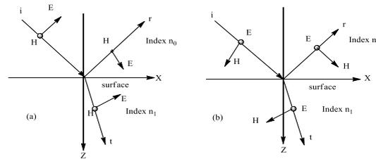
Fig. 1. (a) The positive directions of the electric and magnetic fields for TM mode. (b) The positive directions of the electric and magnetic field for TE mode.
