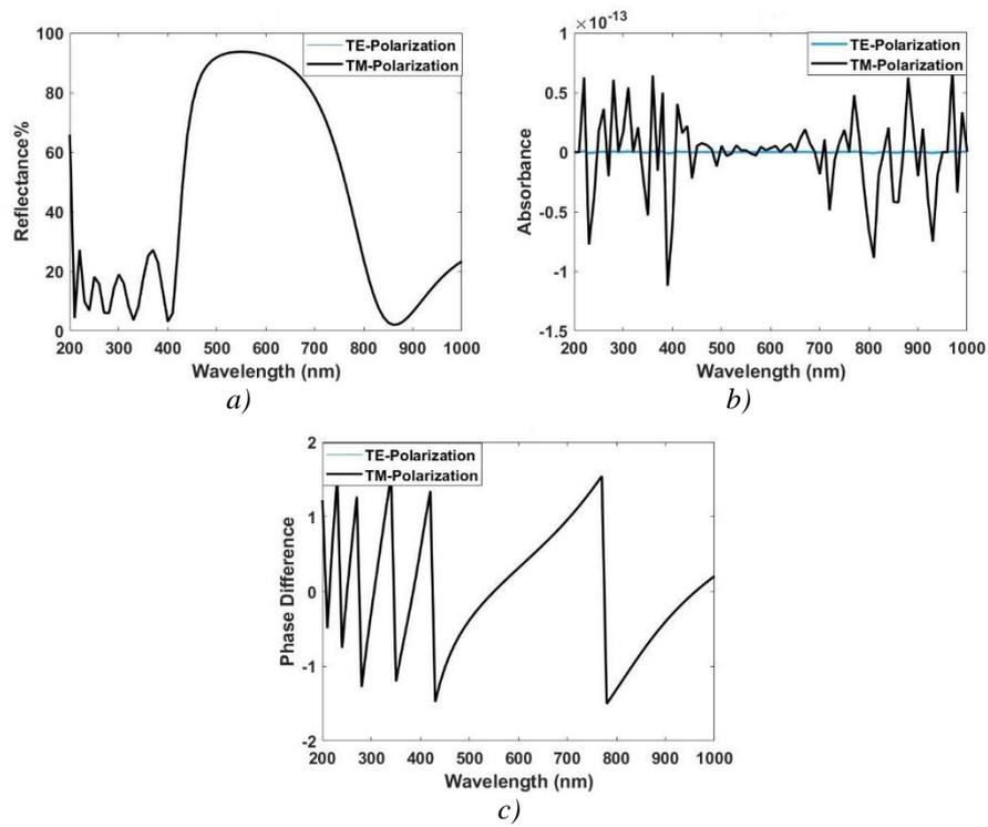
Fig. 6. (a) Reflectance, (b) Absorbance, and (c) Phase Difference as a function of the wavelength for six layers at an incident angle ( $0^\circ$ ).
