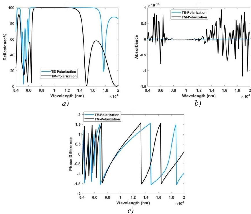
Fig. 4. (a) Reflectance, (b) Absorbance, and (c) Phase Difference as a function of the wavelength for coatings  $n_H = 5.64$ ,  $n_l = 1.44$ , and  $n_s = 5.64$ , for eight layers at an incident angle ( $60^\circ$ ).
