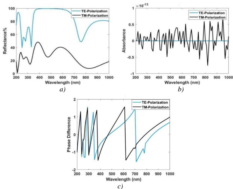
Fig. 8. (a) Reflectance, (b) Absorbance, and (c) Phase Difference as a function of the wavelength at an incident angle ( $80^\circ$ ).
