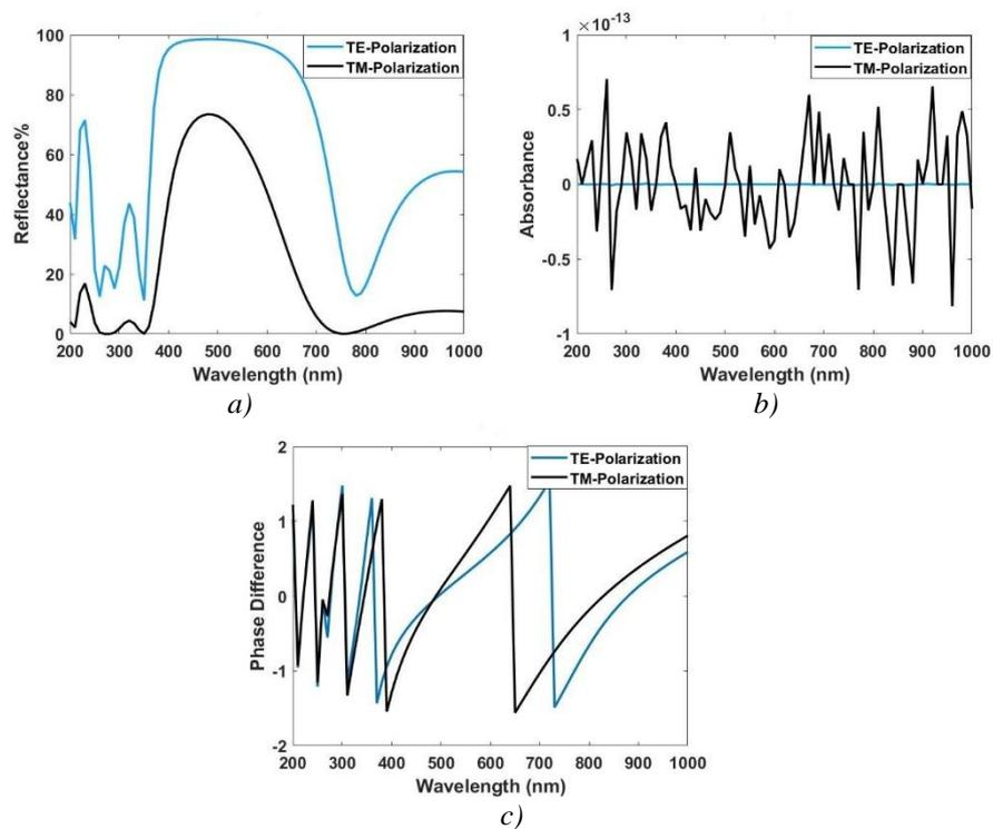
Fig. 7. (a) Reflectance, (b) Absorbance, and (c) Phase Difference as a function of the wavelength for six layers at an incident angle ( $60^\circ$ ).
