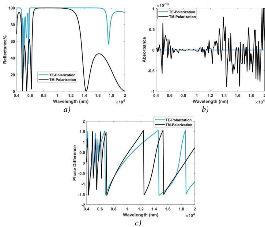
Fig. 5. (a) Reflectance, (b) Absorbance, and (c) Phase Difference as a function of the wavelength for coatings  $n_H = 5.64$ ,  $n_l = 1.44$ , and  $n_s = 5.64$ , for eight layers at an incident angle ( $80^\circ$ ).
