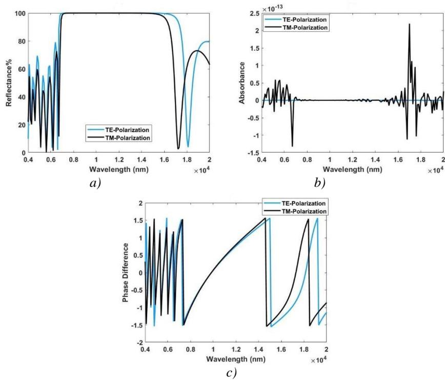
Fig. 3.(a) Reflectance, (b) Absorbance, and (c) Phase Difference as a function of the wavelength for coatings  $n_H = 5.64$ ,  $n_l = 1.44$ , and  $n_s = 5.64$ , for eight layers at an incident angle ( $30^\circ$ ).
