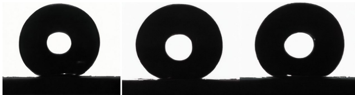
Fig. 5. Contact angle measurements of the three composite film demonstrating excellent waterproof properties.
