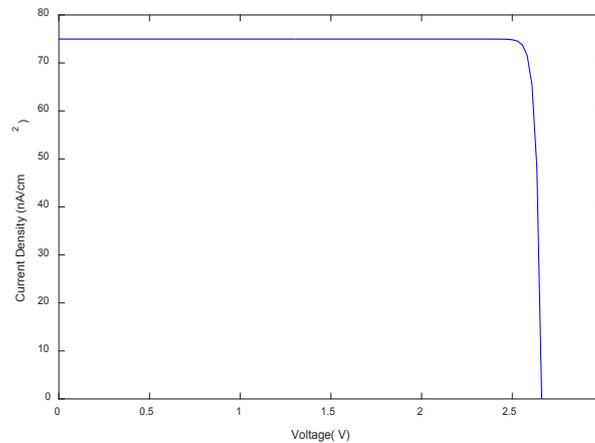
Fig. 4. Current Density voltage for GaN/GaN.
