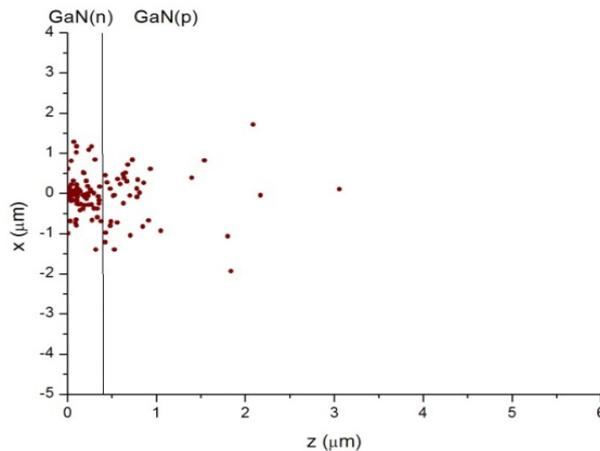
Fig. 2. The distribution of electron-hole pairs generated as a function of depth in GaN for an acceleration energy 17 KeV.
