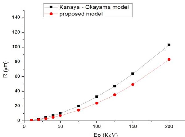
Fig. 1. Stopping range of electrons for GaN as function of acceleration energy.
