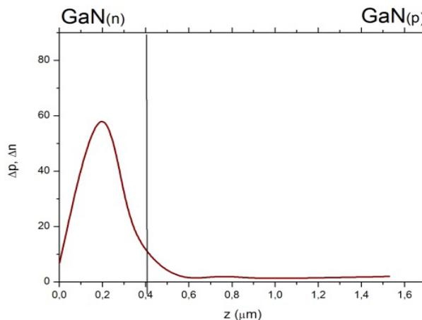
Fig. 3. The distribution of the concentration of electron-hole pairs generated by inelastic collisions of the incident electron in GaN/GaN.
