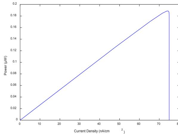
Fig. 5. Current density power (J-P) for GaN/GaN.
