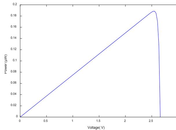
Fig. 6. Power-voltage (P-V) for GaN/GaN.
