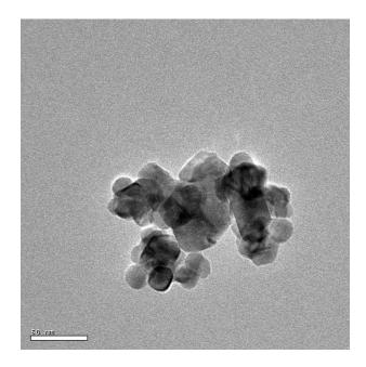
*Fig.4 TEM image of ethylene glycol mediated tin oxide nanoparticles calcined at 400°C.*
