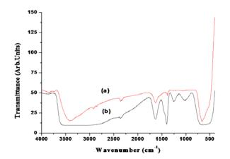
Fig.2 FTIR spectra of tin oxide nanoparticles heat-treated at  $80^{\circ}C(a)$  ethylene glycol (b) water-ethylene glycol mixture as a solvent.
