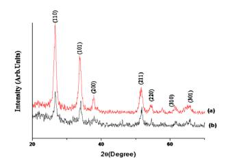
Fig.1 XRD pattern of tin oxide nanoparticles calcined at 400°C by using (a) ethylene glycol (b) water-ethylene glycol mixture as a solvent.
