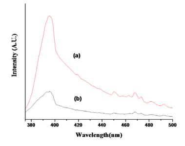
*Fig.6 PL emission spectra of tin oxide nanoparticles calcined at 400°C by using (a) ethylene glycol (b) water-ethylene glycol mixture as a solvent.*
