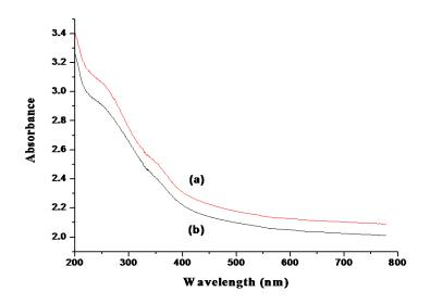
Fig.5 UV-Vis absorption spectra of tin oxide nanoparticles calcined at 400°C by using (a) ethylene glycol (b) water-ethylene glycol mixture as a solvent.
