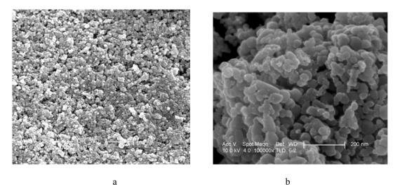
*Fig.3 SEM morphology of tin oxide nanoparticles calcined at 400°C by using (a) ethylene glycol (b) water-ethylene glycol mixture as a solvent.*
