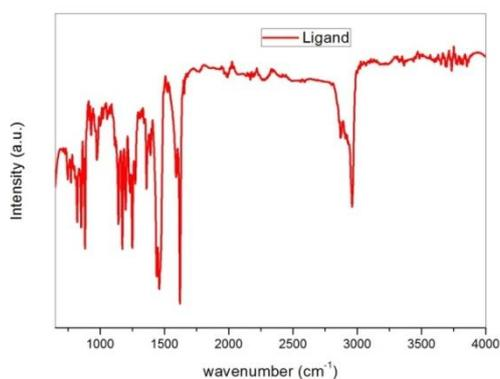
Figure 5a FT-IR spectra for 4,4'-methylene bis (2,6-diethyl) aniline-3,5-di-tert-butylsalicylaldehyde ligand.
