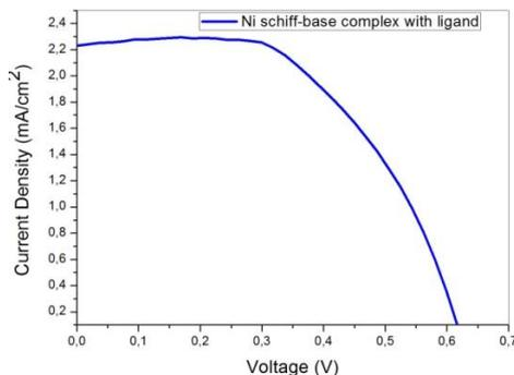
Fig. 7 J-V curve of Ni schiff-base complex containing 4,4'-methylene bis (2,6-diethyl) aniline-3,5-di-tert-butylsalicylaldehyde ligand.
