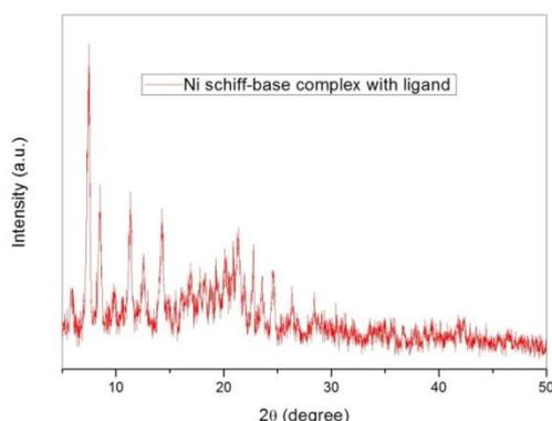
Fig. 3. Diffraction patterns of Ni schiff-base complex with 4,4'-methylene bis (2,6-diethyl) aniline-3,5-di-tert-butylsalicylaldimine ligand
