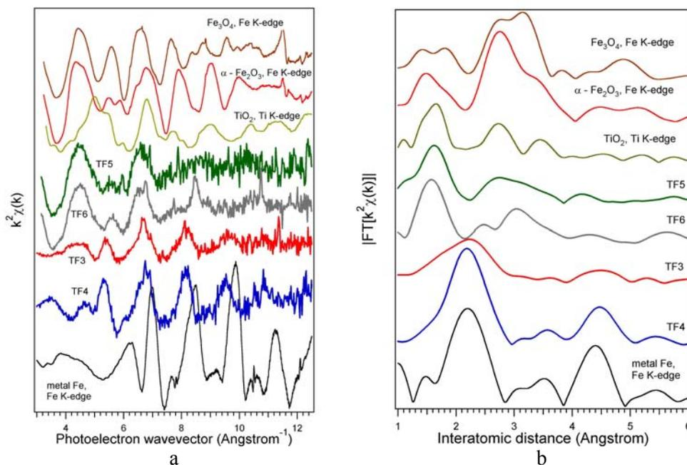
Fig. 4. (a)  $k^2$ -weighted EXAFS spectra  $\Delta\mu/\mu_0$  extracted from the X-ray absorption (Fig. 3); (b) Fourier transforms of the  $k^2$ -weighted EXAFS signal.
