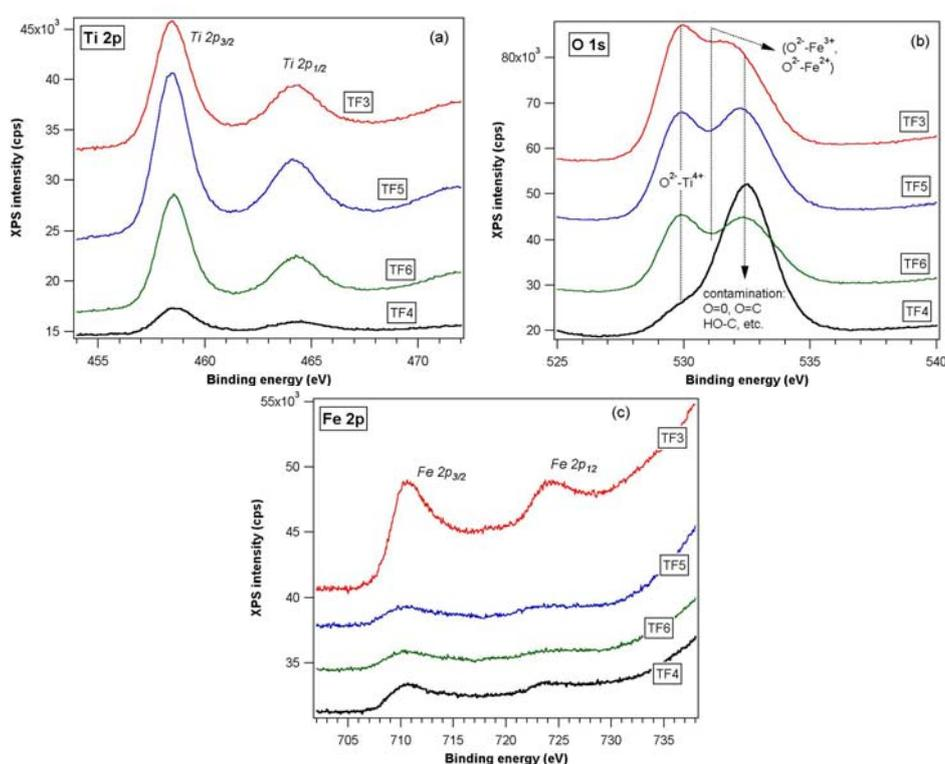
Fig. 2. Electron distribution curves (EDC) obtained by X-ray photoelectron spectroscopy of the Ti 2p levels (a); O 1s levels (b); Fe 2p levels (c).
