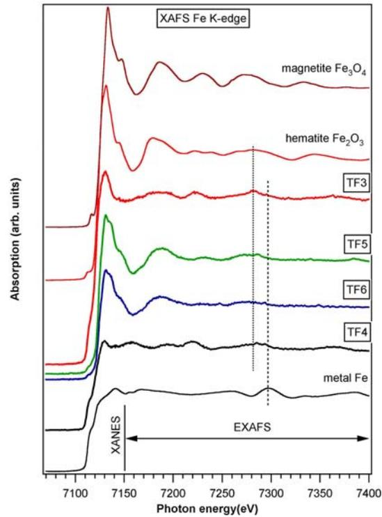
Fig. 3. Fe K-edge X-ray absorption fine structure spectra of samples TF3-6, compared with spectra of reference oxides (hematite  $\text{Fe}_2\text{O}_3$ , magnetite  $\text{Fe}_3\text{O}_4$ ) and of metal Fe. The EXAFS and XANES regions are indicated.
