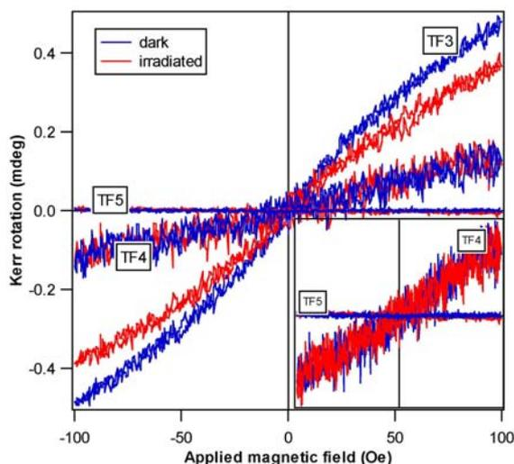
Fig. 1. Magneto-optical Kerr effect (MOKE) loops for various samples. Blue curves: measurements performed in dark, red curves: measurements while irradiating the samples in the optical range.
