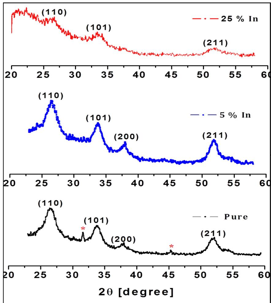
Fig. 1 XRD patterns of pure and In-doped  $\text{SnO}_2$  thin films
