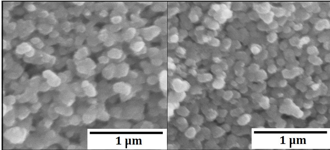
Fig. 2 SEM micrographs of (a) Pure and (b) 5% In-doped  $\text{SnO}_2$  thin films.
