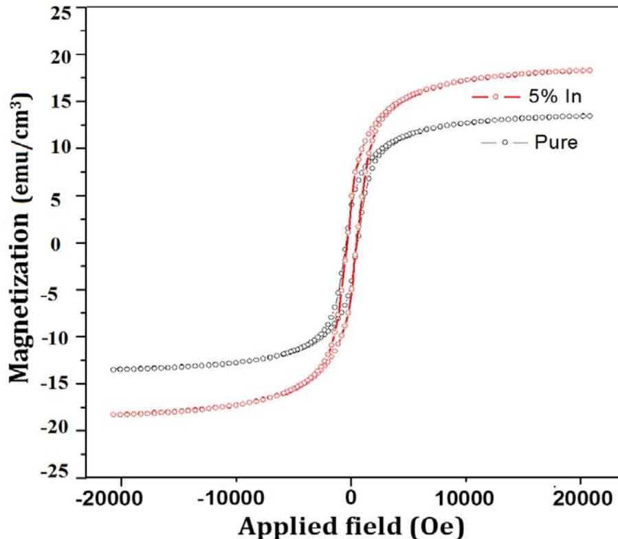
Fig. 4: Magnetization versus magnetic field (M-H) hysteresis loop of pure and 5 % doped-SnO<sub>2</sub> thin films at room temperature.
