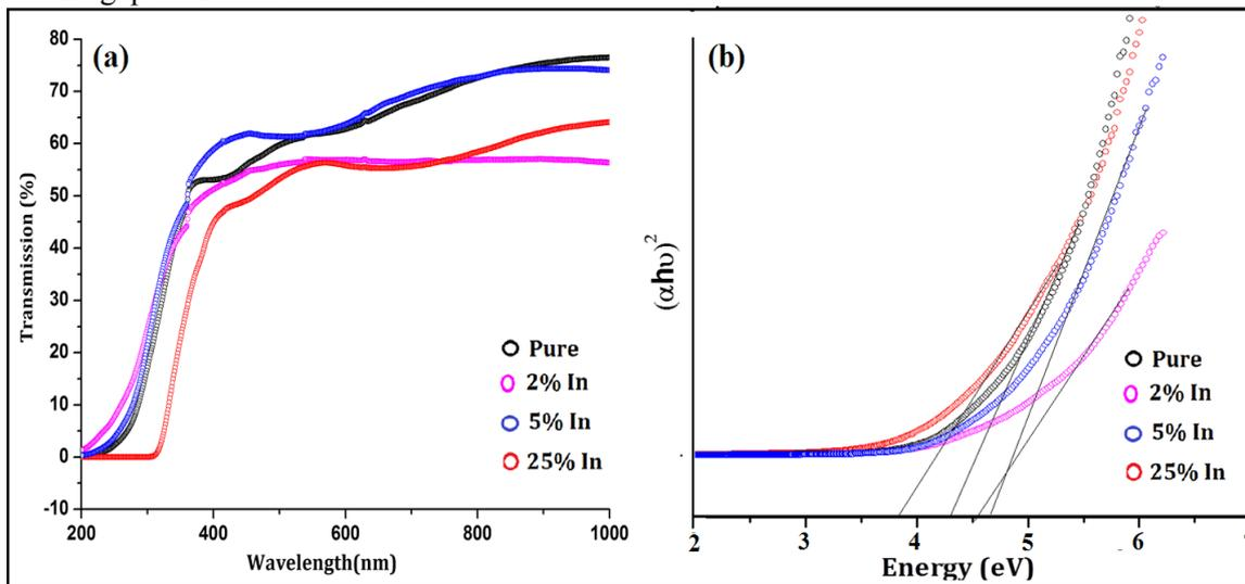
Fig. 3 (a) UV-visible transmission spectra and (b) Tauc's plot of pure and In-doped  $\text{SnO}_2$  thin films.
