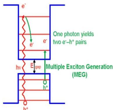
Fig. 14. Multi Exciton Generation Mechanism
