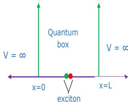
Fig. 5. Exciton in the Quantum Box Model [27]
