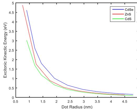
Fig. 6: Excitonic Kinetic Energy versus Dot Radius for CdSe, ZnS and CdS QDs
