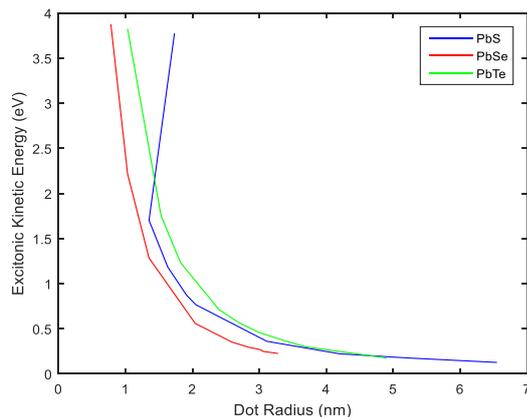
Fig. 8. Excitonic Kinetic Energy versus Dot Radius for PbS, PbSe and PbTe QDs
