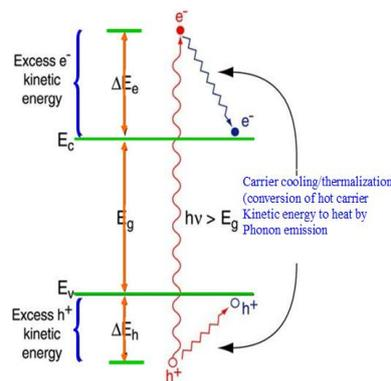
Fig. 2. Hot carrier cooling in semiconductors [10]
