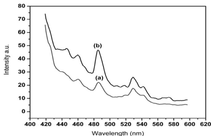
Fig.4 (a, b). The room temperature PL emission of CdS nano crystals on (a) unpolished and (b) chemically polished p-Si(100) substrates.
