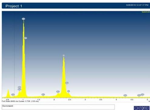
Fig. 5. EDX spectra for Ce-doped ZnS nanoparticles
