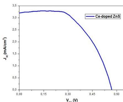
Fig. 7b. Recorded J-V curve for Ce doped ZnS/TiO<sub>2</sub>/FTO structures
