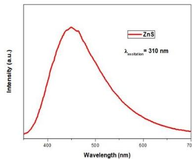
Fig. 4a. The recorded PL spectrum at room temperature for pure ZnS nanoparticles
