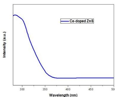
Fig. 2b. The recorded optical absorption spectra for Ce-doped ZnS nanoparticles
