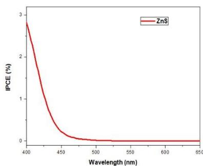
Fig. 6a. The recorded IPCE (%) spectrum at different incident light wavelengths for pure ZnS/TiO<sub>2</sub>/FTO Structure
