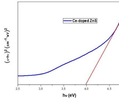
Fig. 3b. The plotted  $(\alpha hv)^2$  vs  $(hv)$  curve for Ce-doped ZnS nanoparticles
