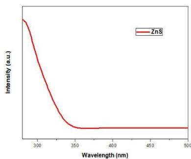
Fig. 2a. The recorded optical absorption spectra for pure ZnS nanoparticles
