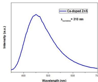
Fig. 4b. The recorded PL spectrum at room temperature for Ce-doped ZnS nanoparticles
