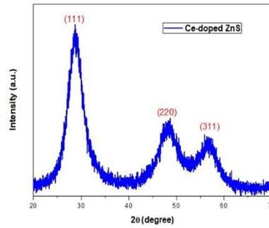
Fig. 1b. The recorded XRD patterns for Ce-doped ZnS nanoparticles
