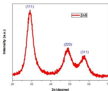
Fig. 1a. The recorded XRD patterns for pure ZnS nanoparticles
