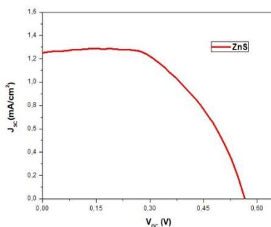
Fig. 7a. Recorded J-V curve for pure ZnS/TiO<sub>2</sub>/FTO structure
