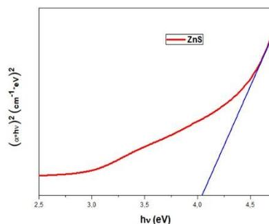
Fig. 3a. The plotted  $(\alpha h\nu)^2$  vs  $(h\nu)$  curve for pure ZnS nanoparticles
