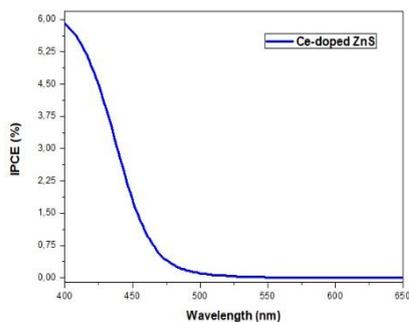
Fig. 6b. The recorded IPCE (%) spectrum at different incident light wavelengths for Ce doped ZnS/TiO<sub>2</sub>/FTO structures
