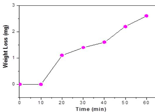
Fig. 2. Weight loss versus etching time for the Si etched by HF.
