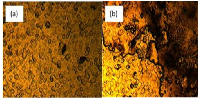
*Fig. 5. Surface morphology of silicon wafer (a) before and (b) after an hour etching in HF/H<sub>2</sub>O solution.*
