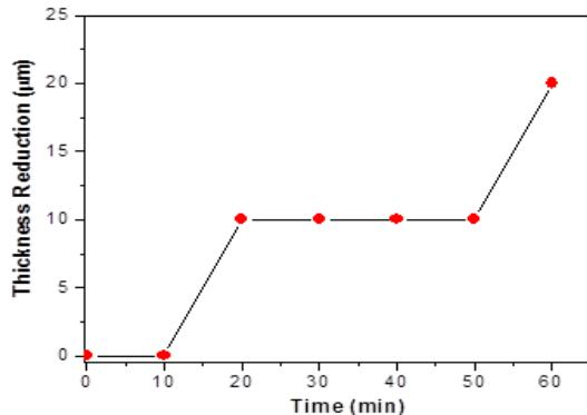
Fig. 1. Thickness reduction versus etching time for the Si immersed in HF.
