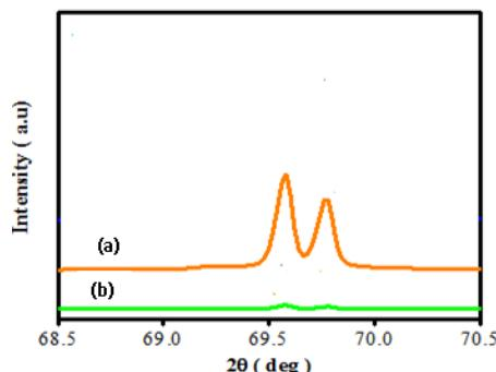
*Fig. 6. XRD pattern of Si (a) before etching and (b) after etching with HF/H<sub>2</sub>O.*
