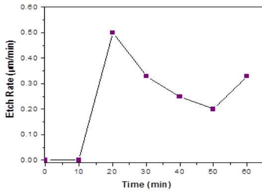
Fig. 3. Etch rate of thickness reduction for the silicon etched by HF.
