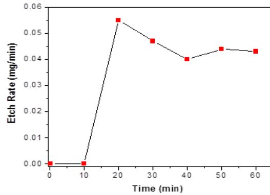
Fig. 4. Etch rate of weigh loss for the silicon etched by HF.
