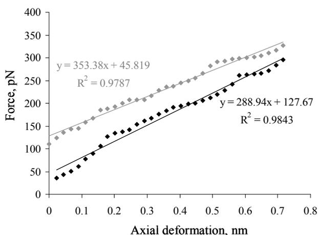
Fig. 3. Force vs. molecular elongation for BMP2 elongation tests performed at a pulling rate of 0.001 nm/ps with a spring constant  $k_s = 3000$  kJ/(mol nm<sup>2</sup>).
