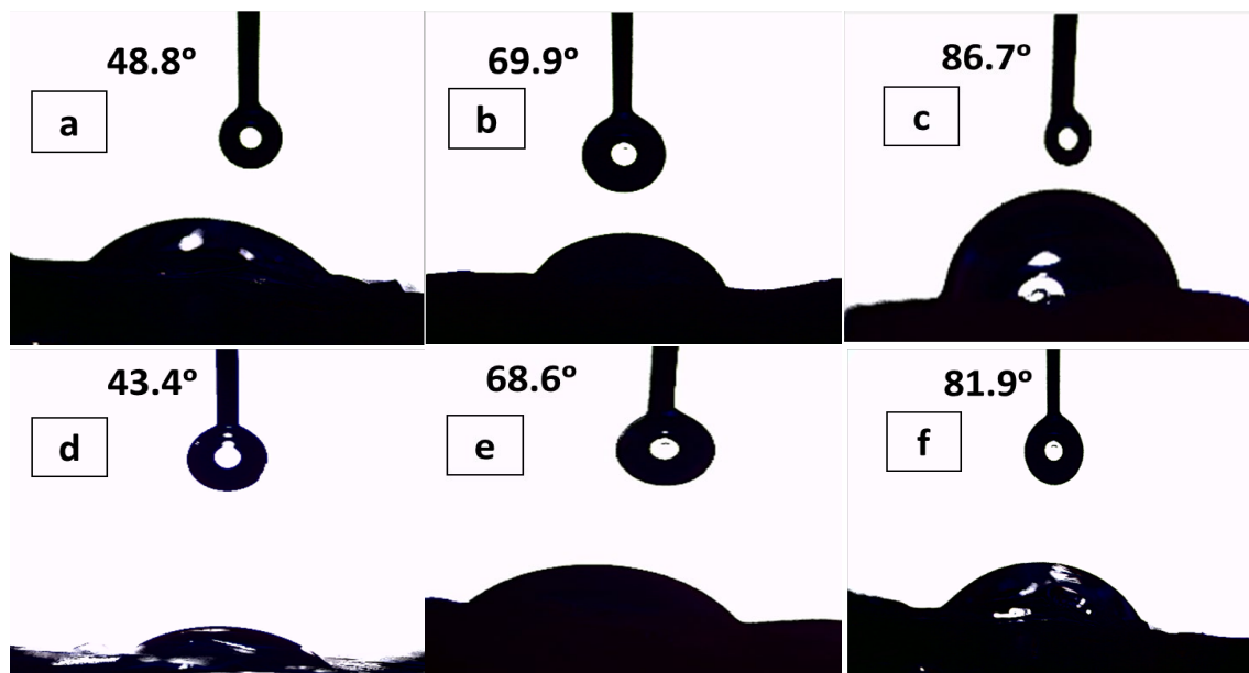
Fig. 10. Contact Angle Images for (a) Pure PVA 2% (b) Pure PVA 5% (c) Pure PVA 10% (d) PVA 2%/BG 2% (e) PVA 5%/BG 2% (f) PVA 10%/BG 2%.
