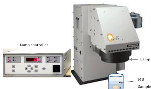
Fig. 2: Sun simulator system (model: Oriel SO12A Solar Simulators)
