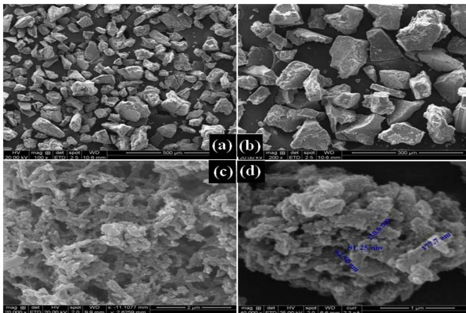
Fig 4. SEM micrographs of (a), (b)  $\text{Cu}_2\text{O}$  nanoparticles, (c) Polyaniline and (d) Polyaniline coated  $\text{Cu}_2\text{O}$  nanoparticles.
