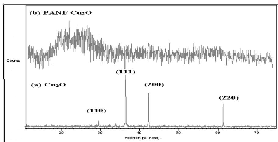
Fig. 3. XRD patterns of (a)  $\text{Cu}_2\text{O}$  nanoparticles and (b) Polyaniline coated  $\text{Cu}_2\text{O}$  nanoparticles.
