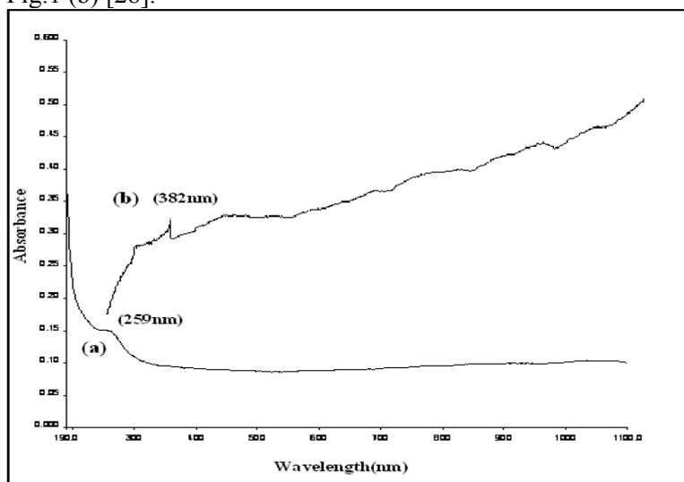
Fig 1. UV-Vis spectrum of (a)  $\text{Cu}_2\text{O}$  nanoparticles and (b) Polyaniline coated  $\text{Cu}_2\text{O}$  nanoparticles.
