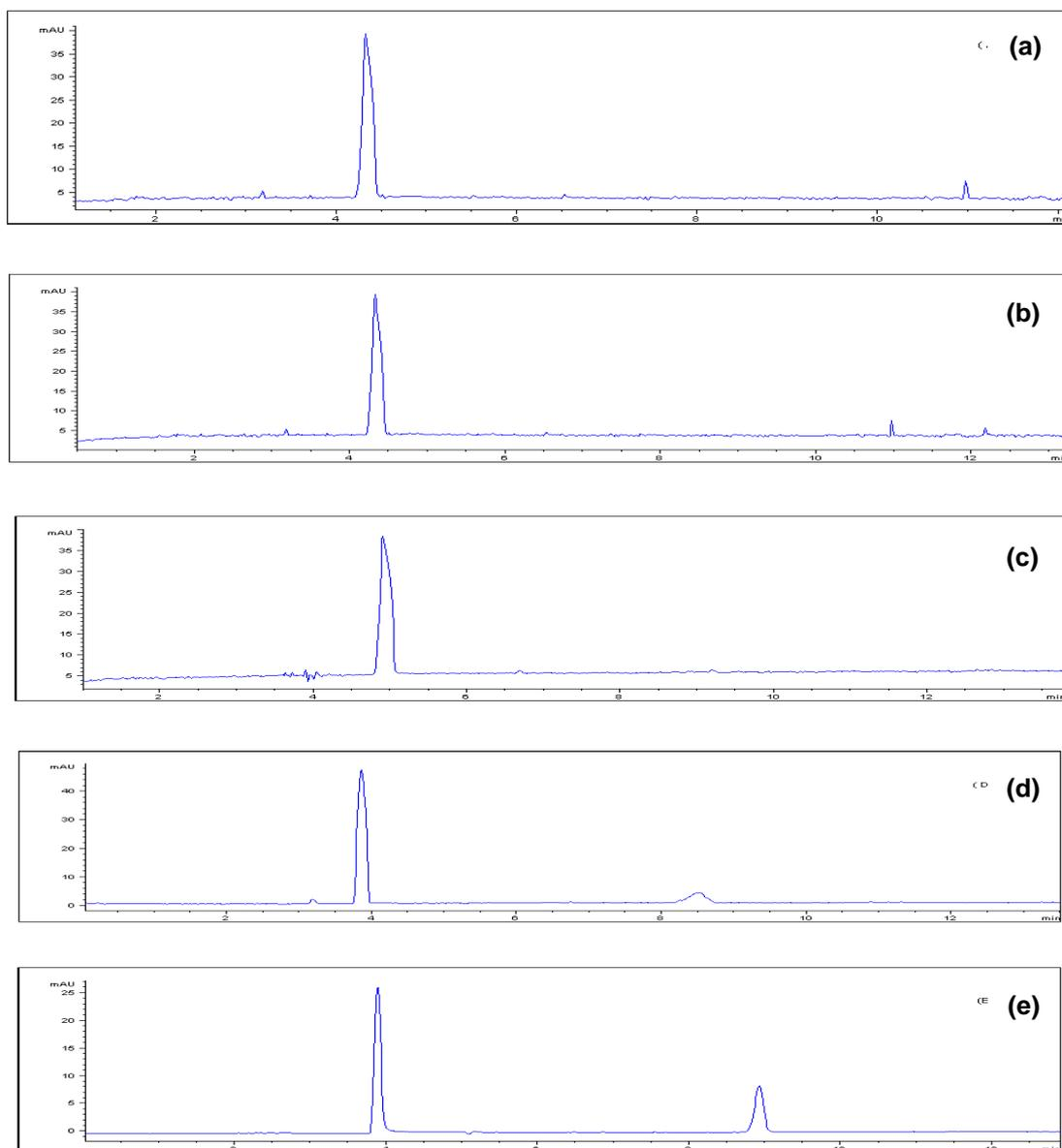
*Fig. 3. Typical electropherograms that have been obtained from stress testing studies of LEN. Panel A is the mixture of standard solution containing LEN (50 µg mL<sup>-1</sup>) and MET (30 µg/mL) that has not been subjected to any stress condition. Panels from B to D are samples that have been subjected to UV irradiation, dry heat, acid hydrolysis, and alkaline hydrolysis, respectively.*
