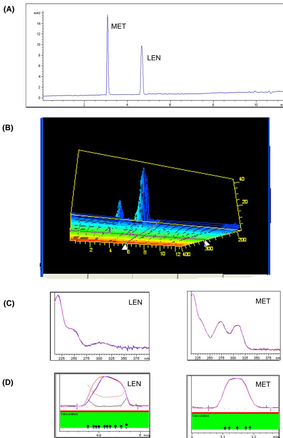
Fig. 2. A typical electropherogram of a standard mixture of  $10 \mu\text{g mL}^{-1}$  of LEN and  $30 \mu\text{g mL}^{-1}$  of MET (A), the corresponding 3D plot (B), their absorption spectra (C), and their corresponding peak purity graphs (D).
