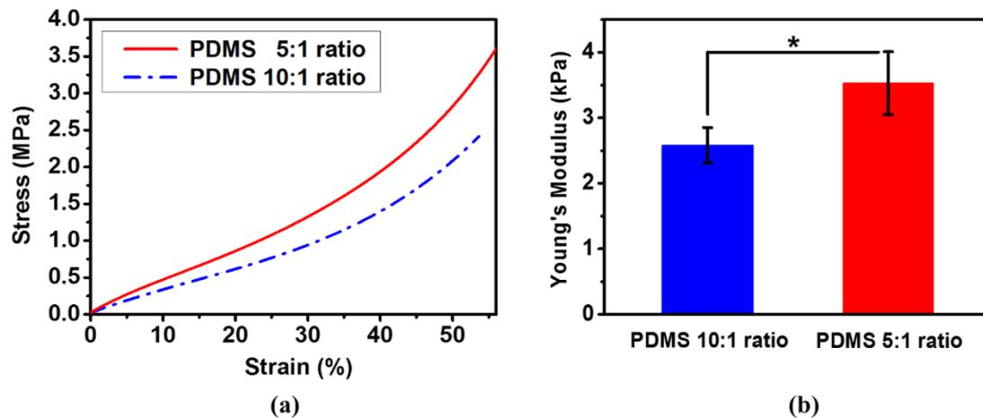
Fig. 1. Compressive strength test. (a) Stress-strain curves and (b) Young's modulus of the fabricated PDMS with 5:1 and 10:1 ratios. (\* $p < 0.001$ ).
