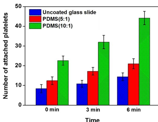
Fig. 4. Comparison of platelets attachment within  $50\mu\text{m} \times 50\mu\text{m}$  area on the surfaces of uncoated, 5:1 PDMS-coated, and 10:1 PDMS-coated glass slides as a function of time (0, 3, and 6 minutes).
