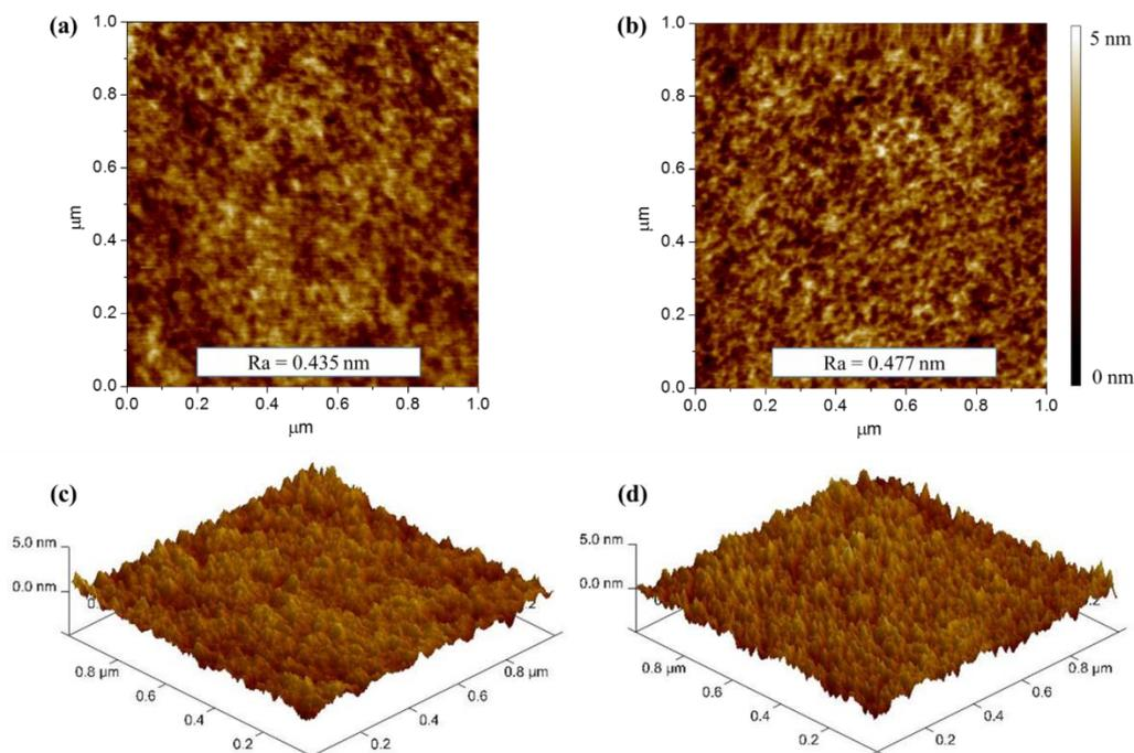
Fig. 2. AFM surface images of two different ratios of PDMS. (a) & (c) PDMS with a 5:1 ratio; (b) & (d) PDMS with a 10:1 ratio.
