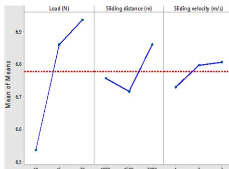
Fig. 11. Mean plot for wear rate.
