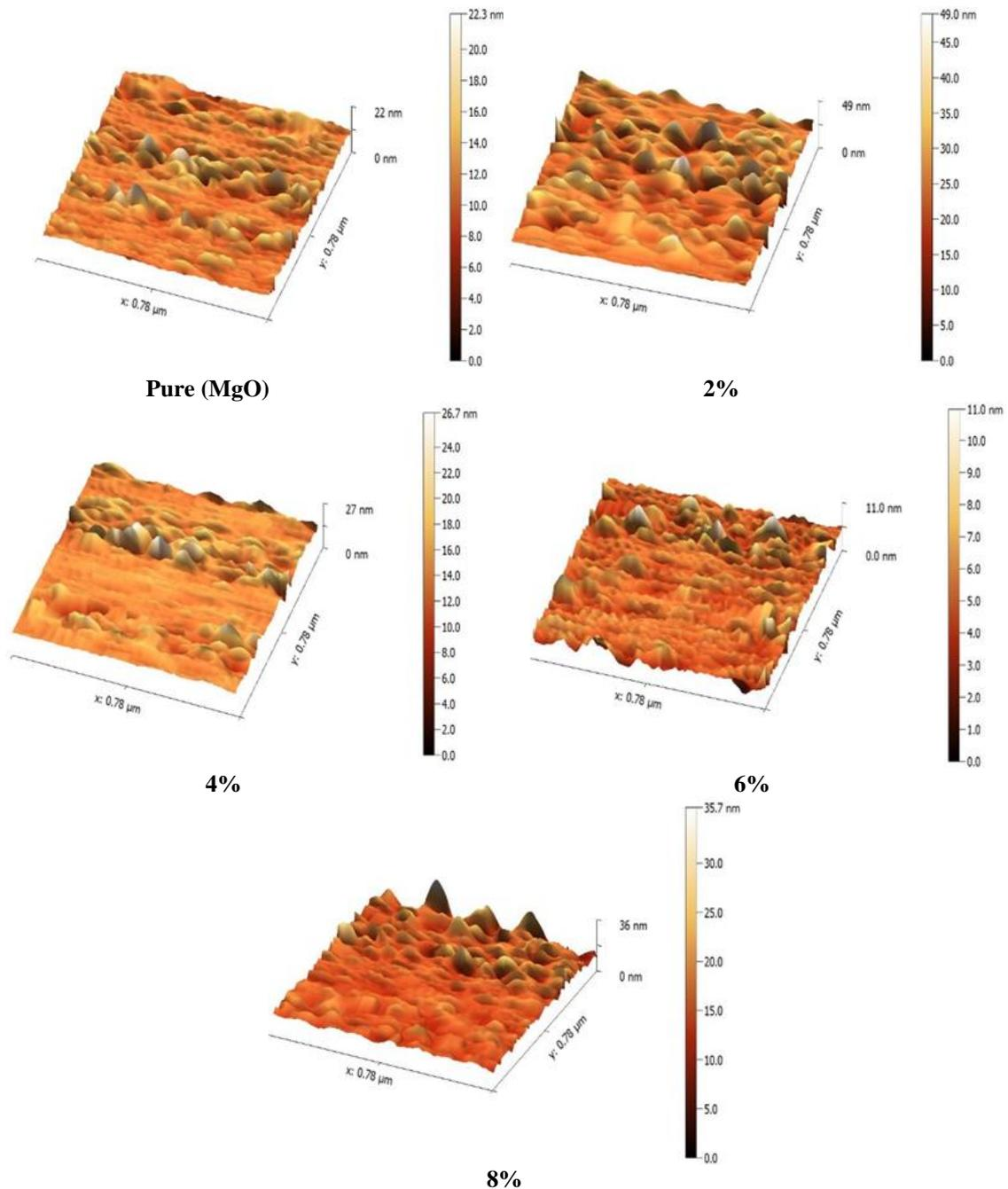
Fig. 1. AFM images of  $\text{MgO}_{1-x}\text{ZnS}_x$  films.
