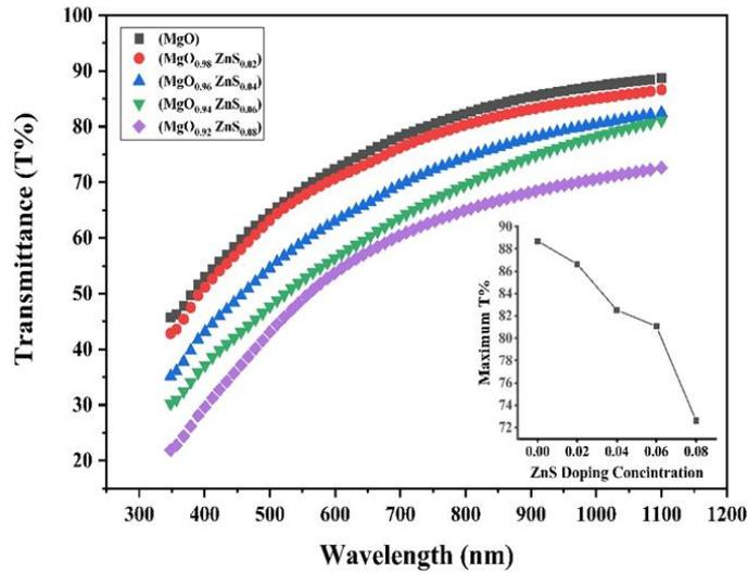
Fig. 3. Transmittance spectra of  $(MgO_{1-x}ZnS_x)$  thin films. Inset figure shows the maximum transmittance with  $(ZnS)$  doping Concentration.
