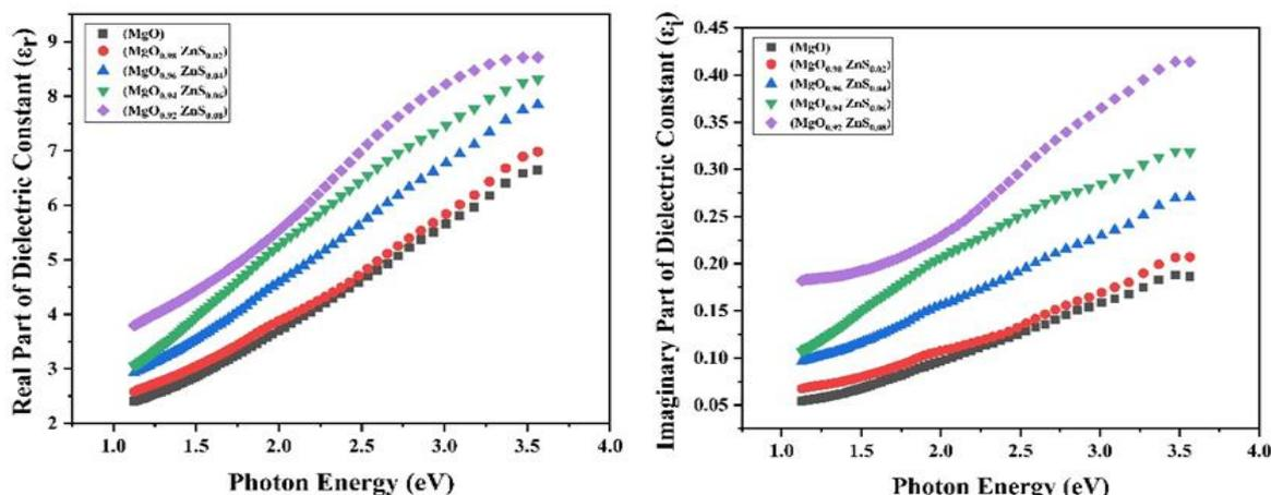
Fig. 9. Real Part of Dielectric Constant and Imaginary Part of Dielectric Constant of  $(MgO_{1-x}ZnS_x)$  thin films.
