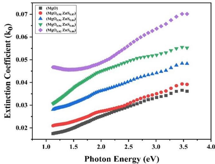
Fig. 7. Extinction Coefficient of  $MgO_{1-x}ZnS_x$  thin films.
