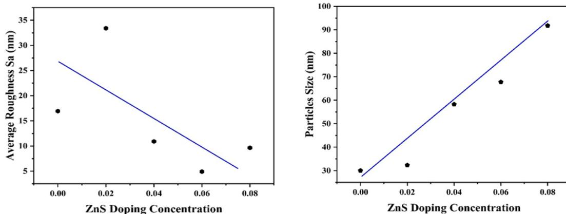
Fig. 2. Average roughness and particle size of  $MgO_{1-x}ZnS_x$  films.
