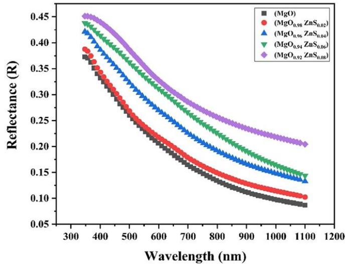
Fig. 4. Reflectance of  $(MgO_{1-x}ZnS_x)$  thin films.
