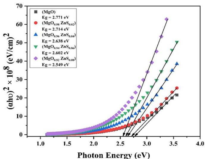
Fig. 6. Energy Gap of (MgO<sub>1-x</sub>ZnS<sub>x</sub>) thin films.
