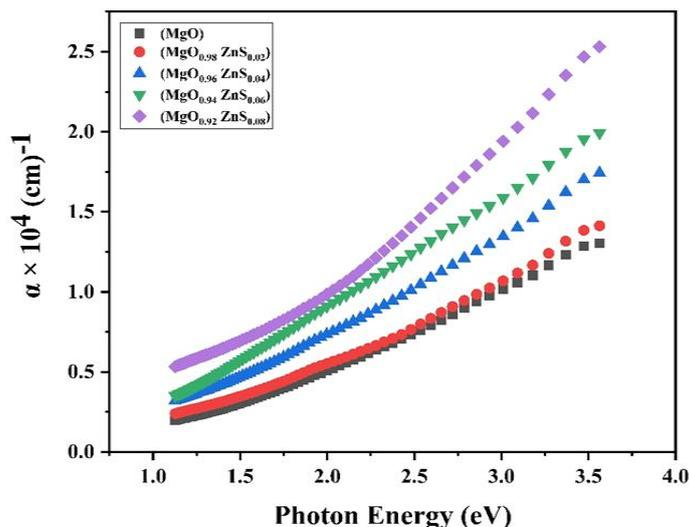
Fig. 5. Absorption Coefficient of (MgO<sub>1-x</sub>ZnS<sub>x</sub>) thin films.
