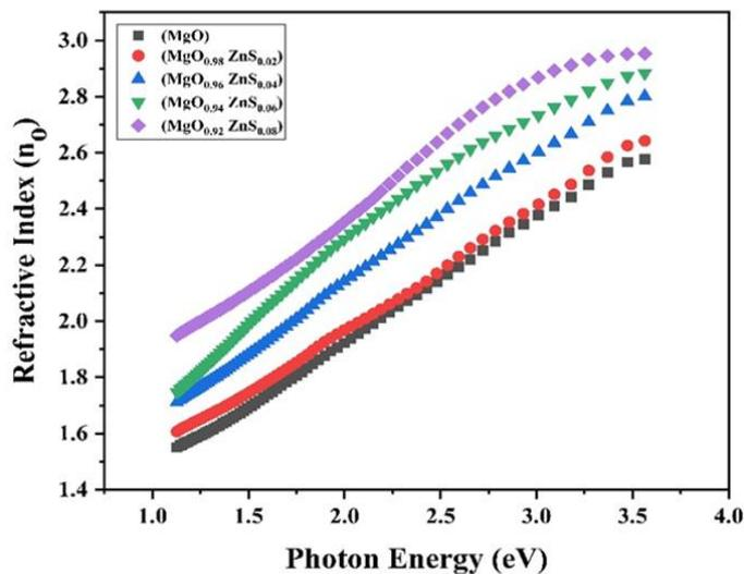
Fig. 8. Refractive Index of  $(MgO_{1-x}ZnS_x)$  thin films.
