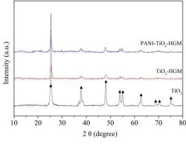
Fig. 1. XRD patterns of different materials
