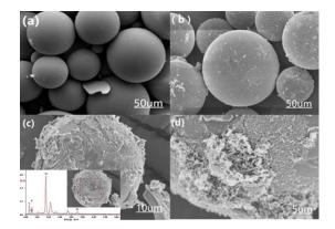
Fig. 3. SEM images of materials: (a) TiO<sub>2</sub>, (b), (c), (d) different size of PTH and EDX spectrum
