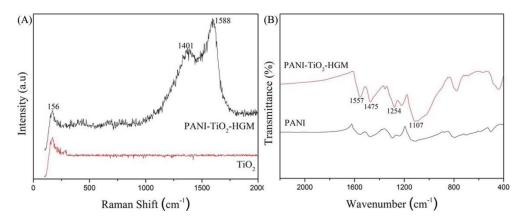
Fig. 2. (A) Raman spectra of TiO<sub>2</sub> and PTH. (B) FT-IR spectra of PANI and PTH
