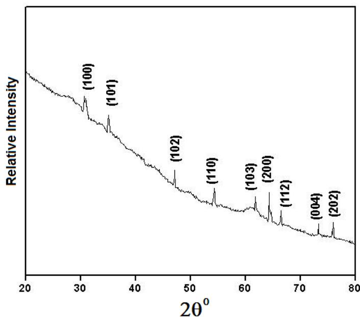
Fig. 1 XRD pattern for a typical CoS thin film.
