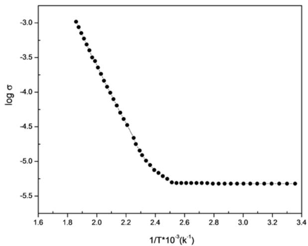
Fig. 3 Variation of  $\log \sigma$  with  $1/T$  for CoS thin film.
