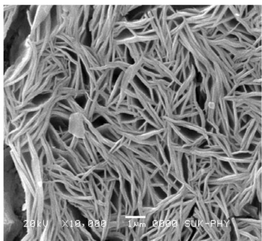
Fig. 4 SEM micrograph of a typical CoS thin film.
