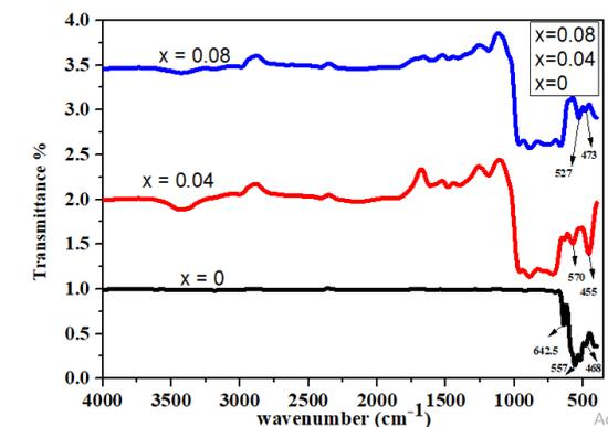
Fig. 3. FT-IR Analysis of  $Sr_{1-x}Cr_xCo_2Fe_{16}O_{27}$  hexagonal ferrite at  $x=0, x=0.04, x=0.08$ .
