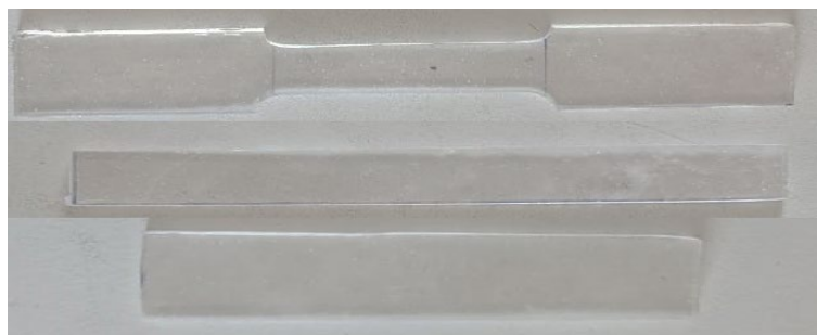
Fig. 2. Tensile , Flexural and Impact Specimens of MWCNT 's and Al_2O_3 Reinforced Epoxy Hybrid Composites
