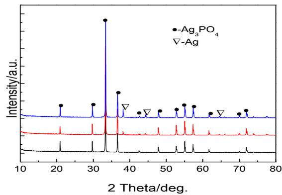
Fig. 2. XRD pattern of nanometer metal Ag modified silver phosphate by precipitation method.
