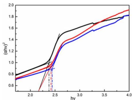
Fig. 6. Forbidden band width map of  $\text{Ag}_3\text{PO}_4$  samples with different Ag loadings.
