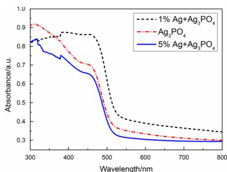
Fig. 5. UV-vis DRS spectra of  $\text{Ag}_3\text{PO}_4$  samples with different Ag loadings.
