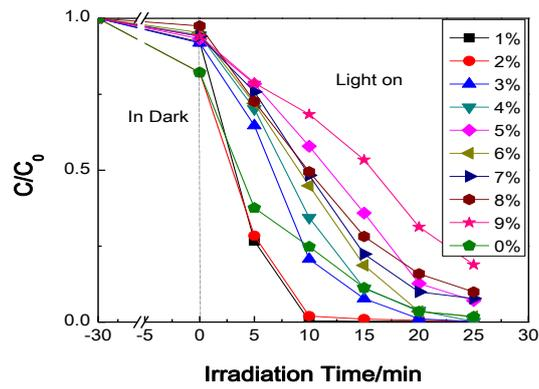
Fig. 1. Photodegradation curve of nanometer metal Ag modified silver phosphate by precipitation method.
