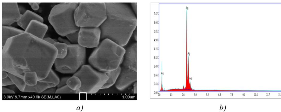
Fig. 3. Scanning electron microscopy and EDS map of Ag/  $Ag_3PO_4$  samples.
