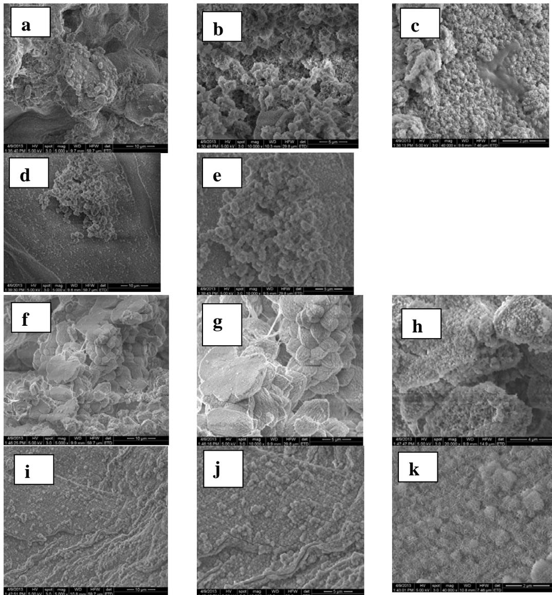
Fig. 6 SEM images of the composite materials soaked in SBF for 14 days:
