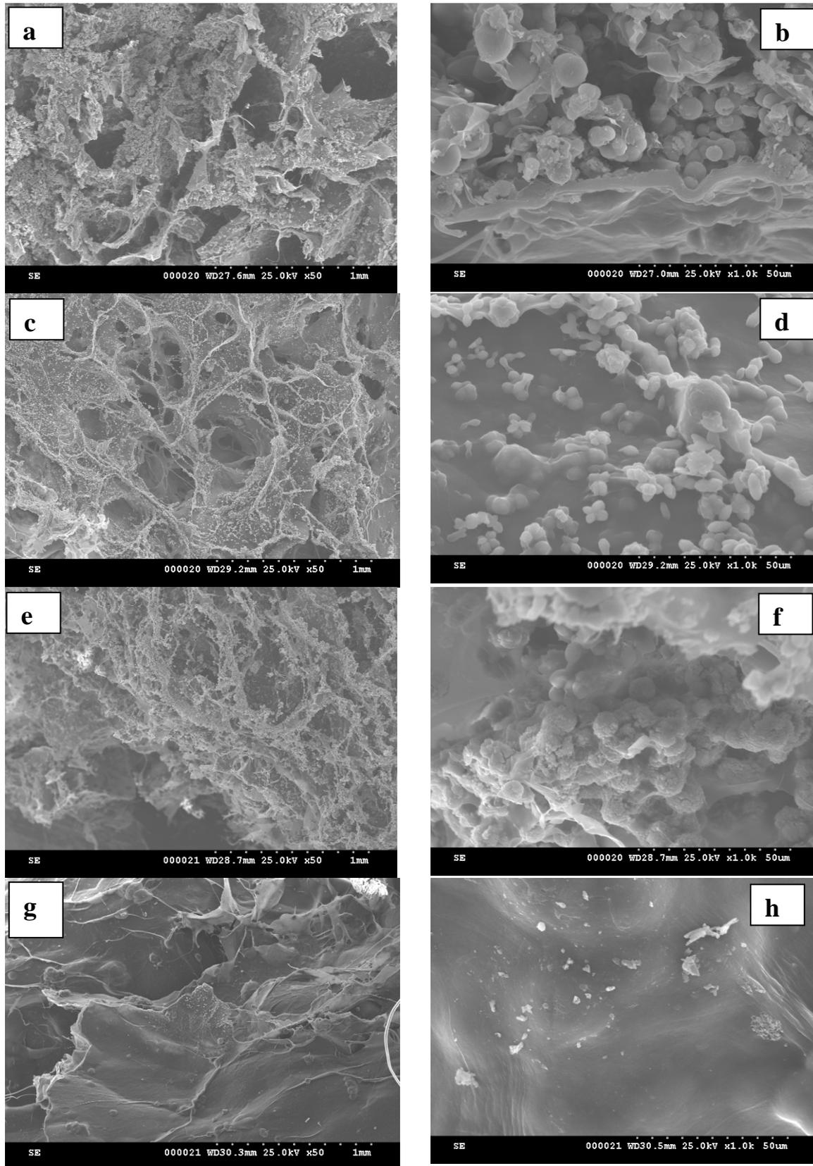
Fig. 4 SEM images of the composite materials: (a, b) MC1, (c, d) MC2, (e, f) MC3 and (g, h) MC4.
