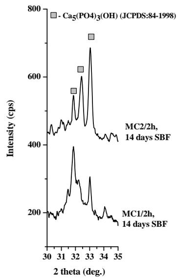
Fig. 5 The XRD patterns of MC1 and MC2 soaked in SBF for 14 days.
