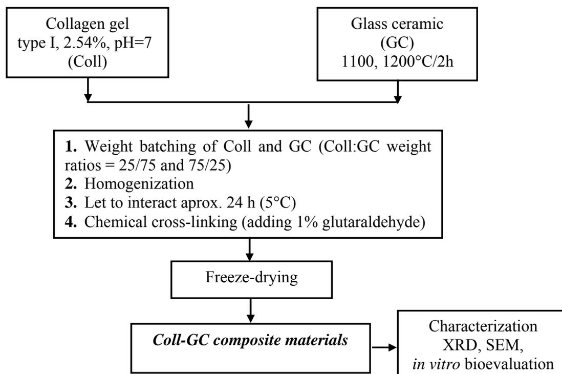
Fig. 1 Scheme of the synthesis of Coll/GC composite materials.
