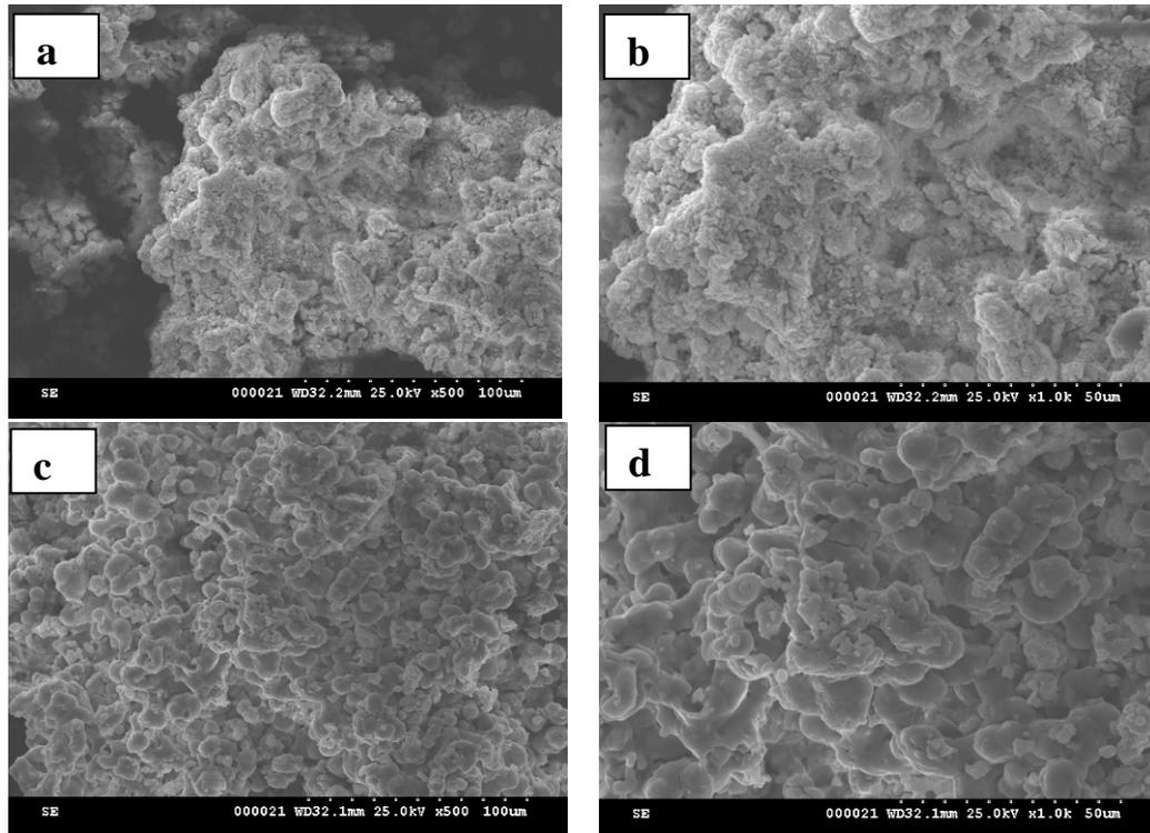
Fig. 3 SEM images of glass ceramic powders obtained at: (a,b) 1100°C/2h and (c,d) 1200°C/2h.
