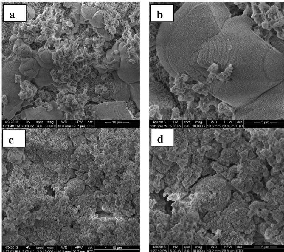
Fig. 7 SEM images of the glass ceramics soaked in SBF for 14 days: (a, b) 1100°C/2h and (c, d) 1200°C/2h.
