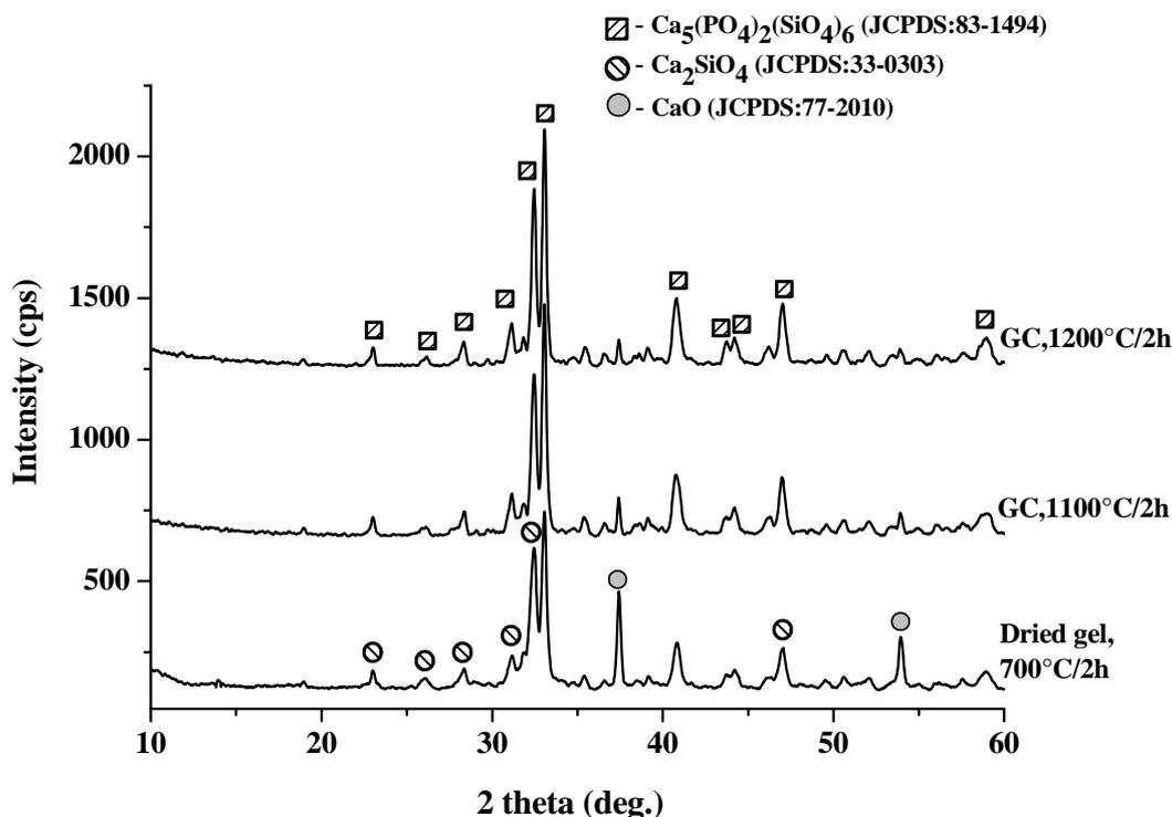
Fig. 2 The XRD patterns of the dried gel thermal treated at 700°C for 2h and glass ceramic powders (1100°C/2h and 1200°C/2h).
