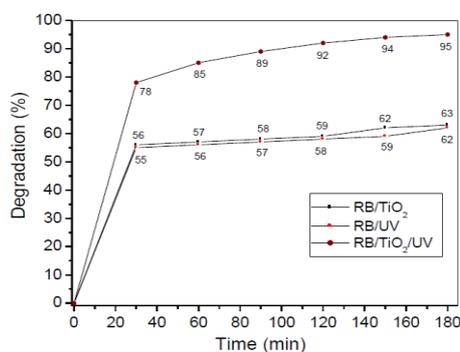
Fig. 4. Degradation efficiency of RB dye solution at different conditions.
