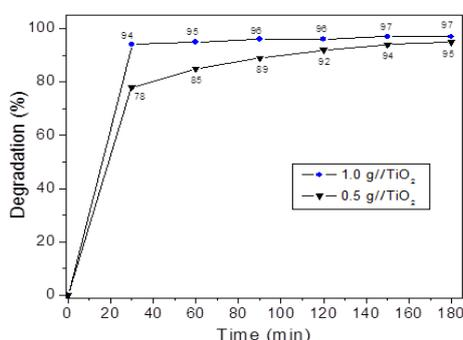
Fig. 5. Degradation efficiency of RB dye solution at different TiO<sub>2</sub> concentrations.
