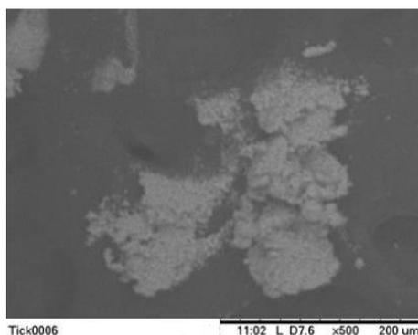
Fig. 3. Surface morphology of  $\text{TiO}_2$  particles.
