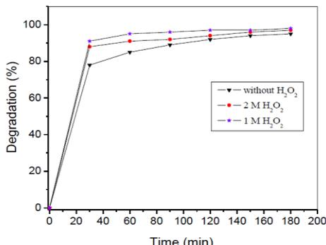
Fig. 6. Degradation efficiency of RB with the addition of different  $\text{H}_2\text{O}_2$  concentrations.
