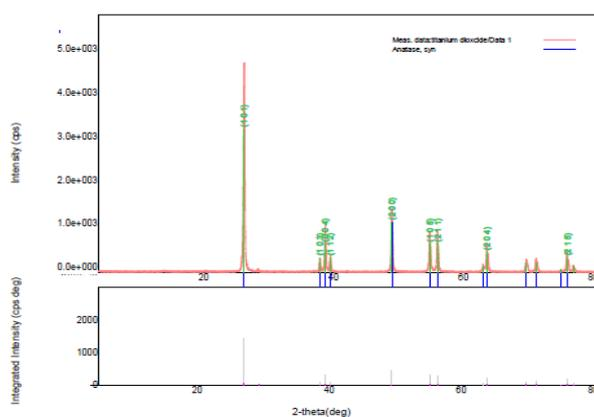
Fig. 2. XRD pattern of as-received  $\text{TiO}_2$ .
