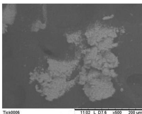
Fig. 3. Surface morphology of  $\text{TiO}_2$  particles.
