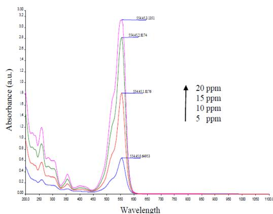
Fig. 1. Absorption spectra of RB solutions at different concentrations.
